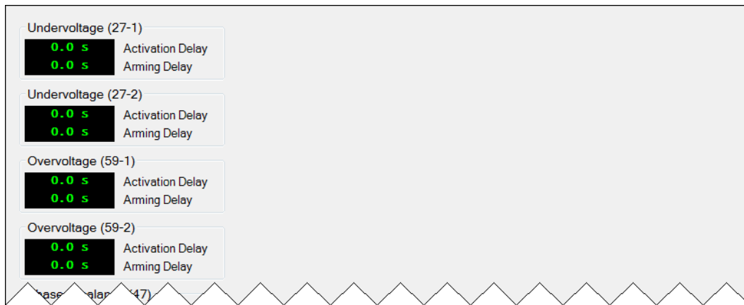
Figure 4-120. Generator Protection Timers
