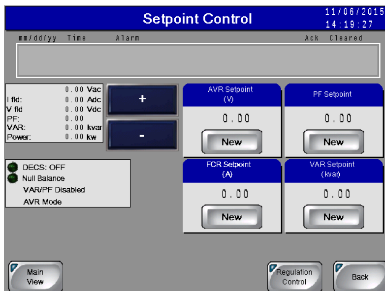
Figure 4-23. Setpoint Control Screen
