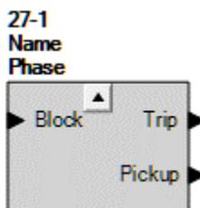
Figure 19-1. Undervoltage Element Logic Block
