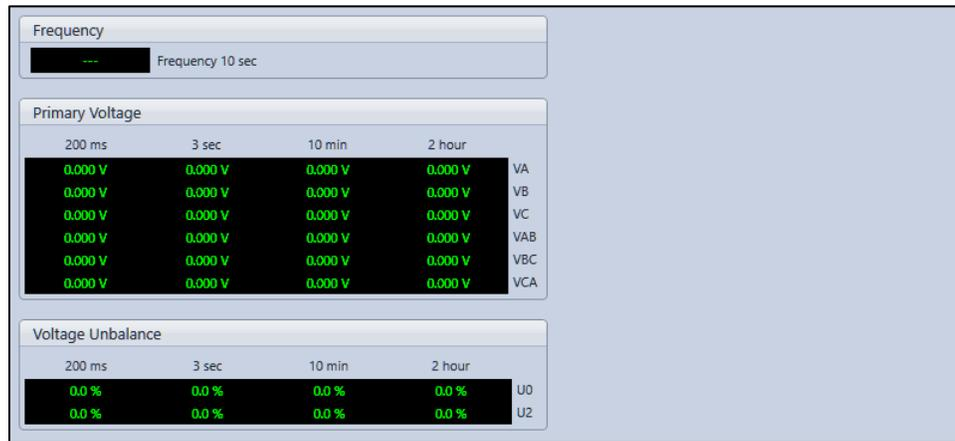
Figure 10-13. Power Quality, Voltage Metering
