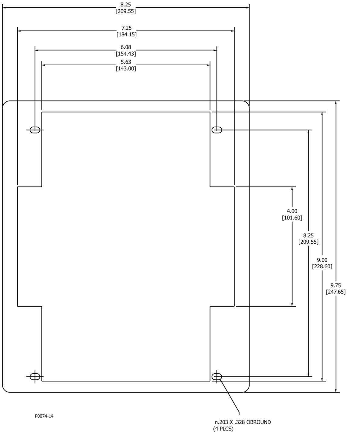
Figure 3-7. Multilin 345/745 Mounting Plate (Basler P/N: 9424200073) – Part 1 of 2
