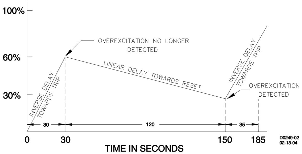
Figure 17-5. Inverse Time Delay and Reset Time
