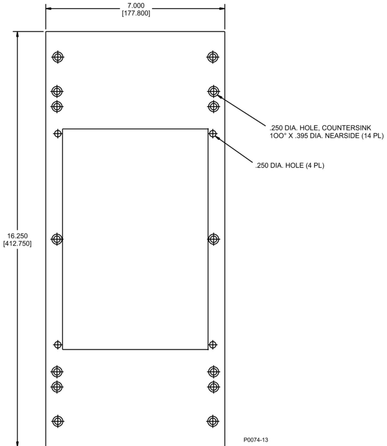
Figure 3-6. GE M1/M2 Adapter Plate (Basler P/N: 9108551029)
