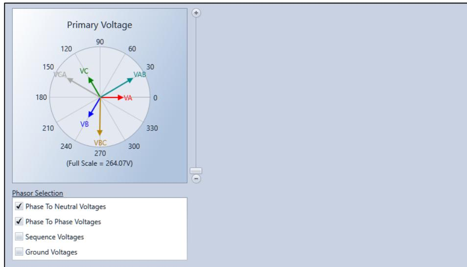
Figure 14-3. Primary Voltage Phasors Metering Screen
