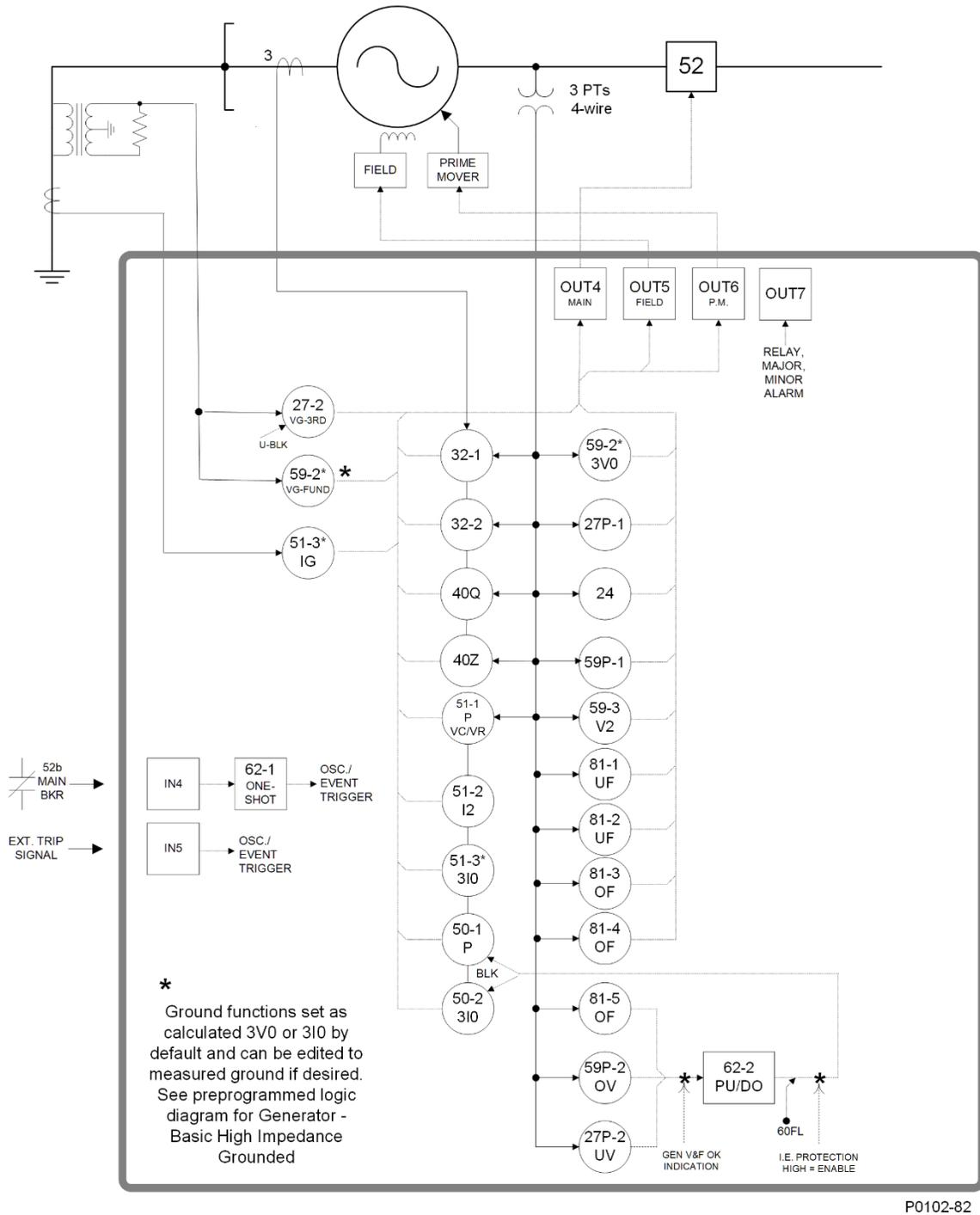
Figure 6-2. Generator - Basic High Impedance Grounded One-Line
