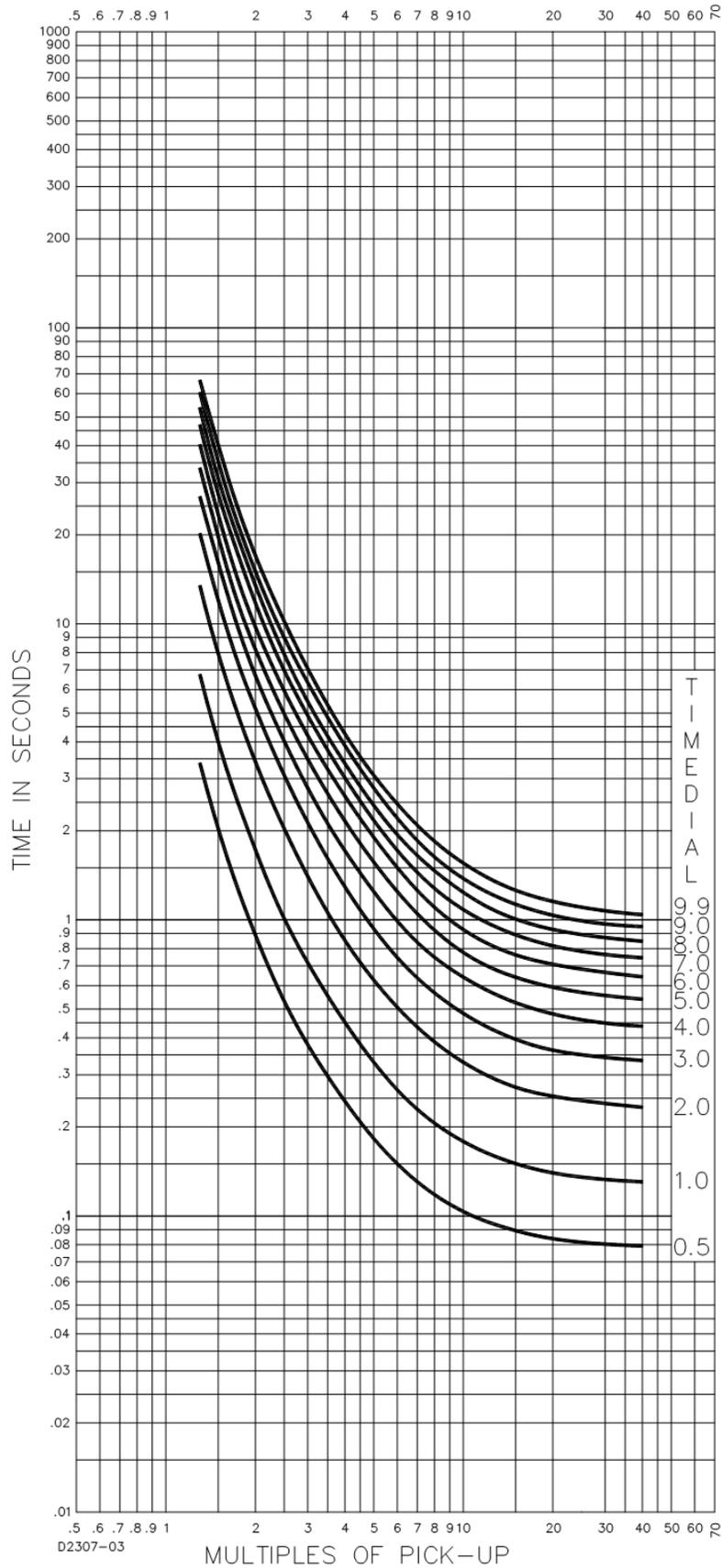
Figure 56-17. Time Characteristic Curve V2, Very Inverse (Similar to GE IAC-53)
