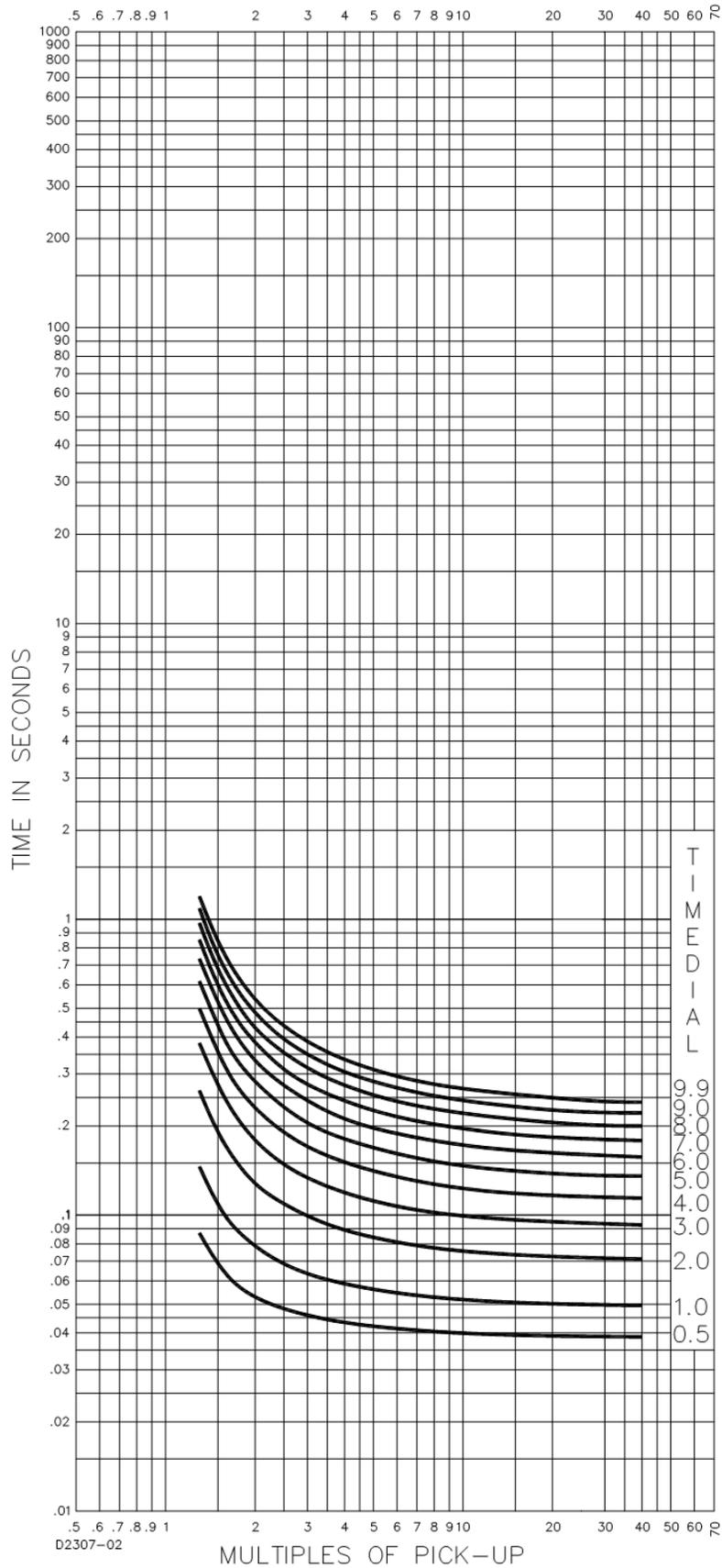
Figure 56-6. Time Characteristic Curve S2, Short Inverse (Similar To GE IAC-55)
