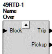
Figure 26-1. Resistance Temperature Detector Element Logic Block
