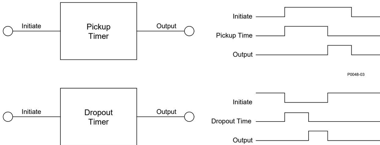
Figure 51-3. Pickup and Dropout Timer Logic Blocks
