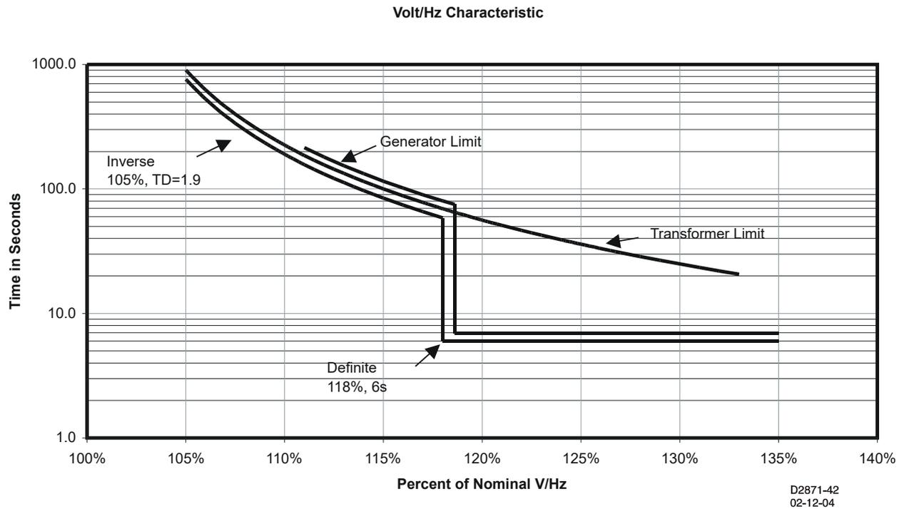
**Figure 17-3. Time Shown on Vertical Axis**
