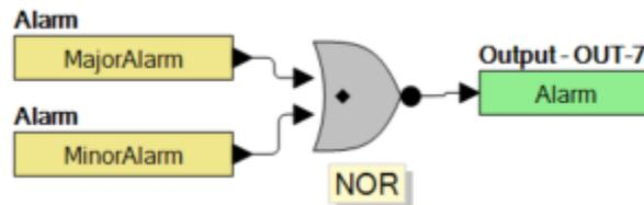
Figure 10-33. Alarm Logic
