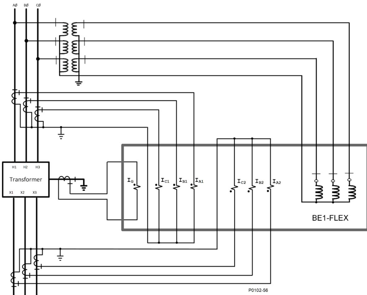
Figure 5-6. Typical AC Connections for Transformer
