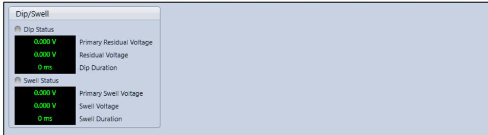
Figure 10-15. Power Quality, Dip/Swell Metering
