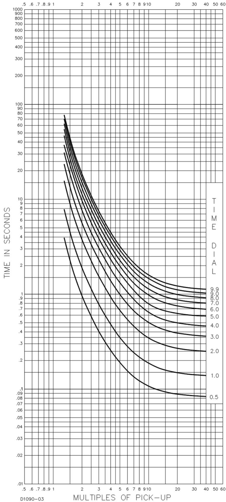
Figure 56-16. Time Characteristic Curve V1, Very Inverse (Similar to ABB CO-9)
