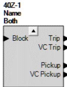
Figure 23-1. Loss of Excitation - Impedance Based Element Logic Block
