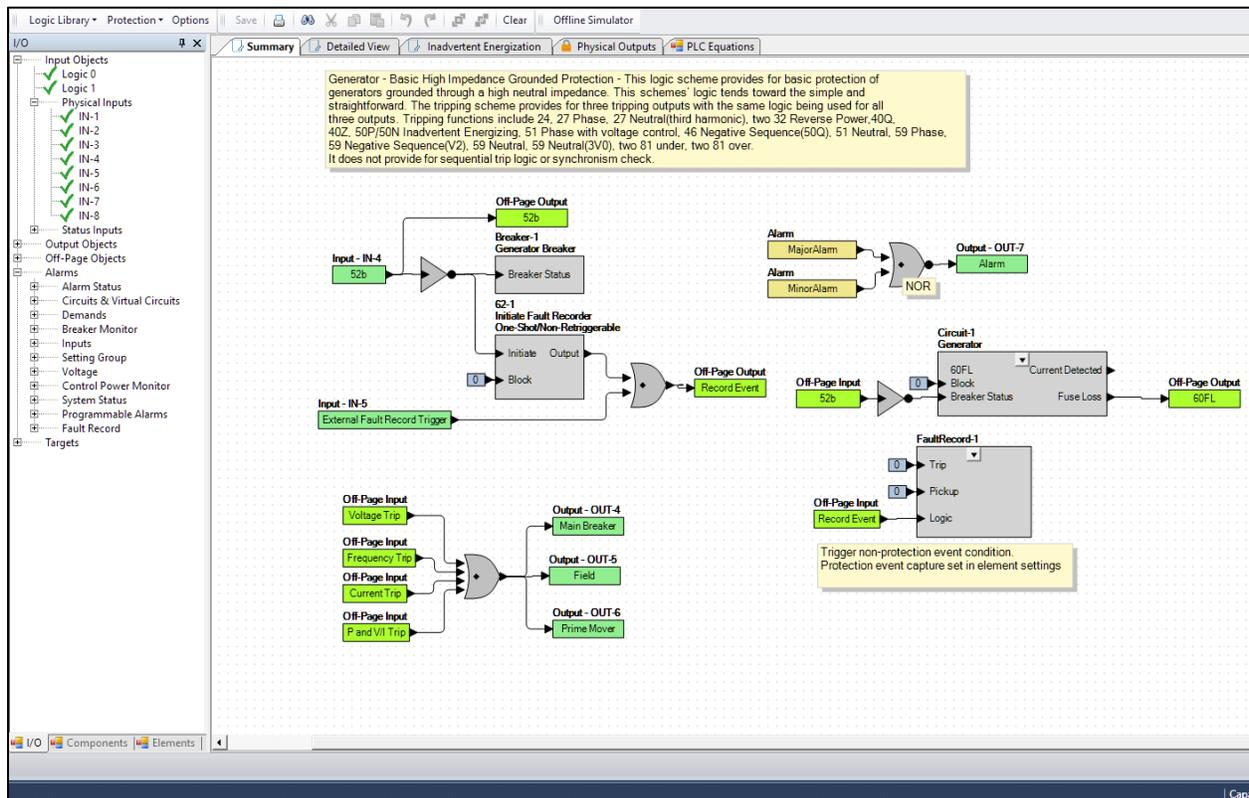
Figure 6-1. Generator - Basic High Impedance Grounded Logic
