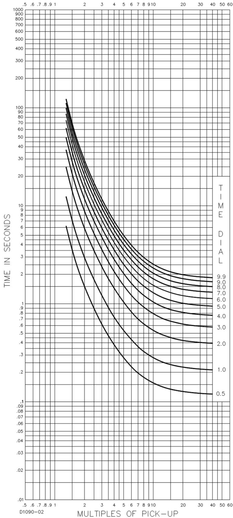
Figure 56-9. Time Characteristic Curve I1, Inverse Time (Similar to ABB CO-8)
