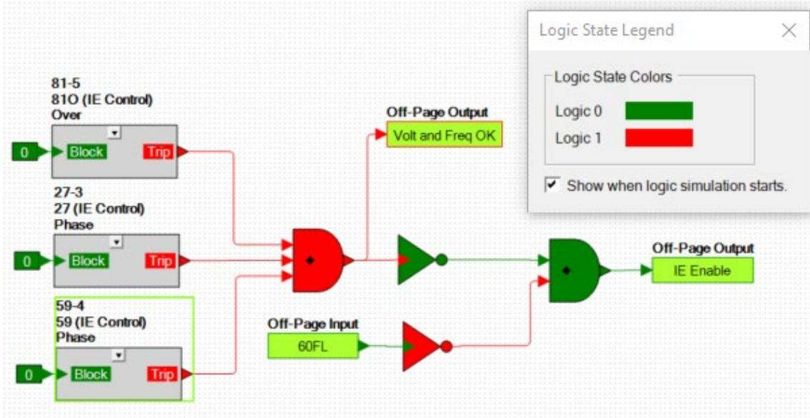
Figure 51-4. Offline Logic Simulator Example
