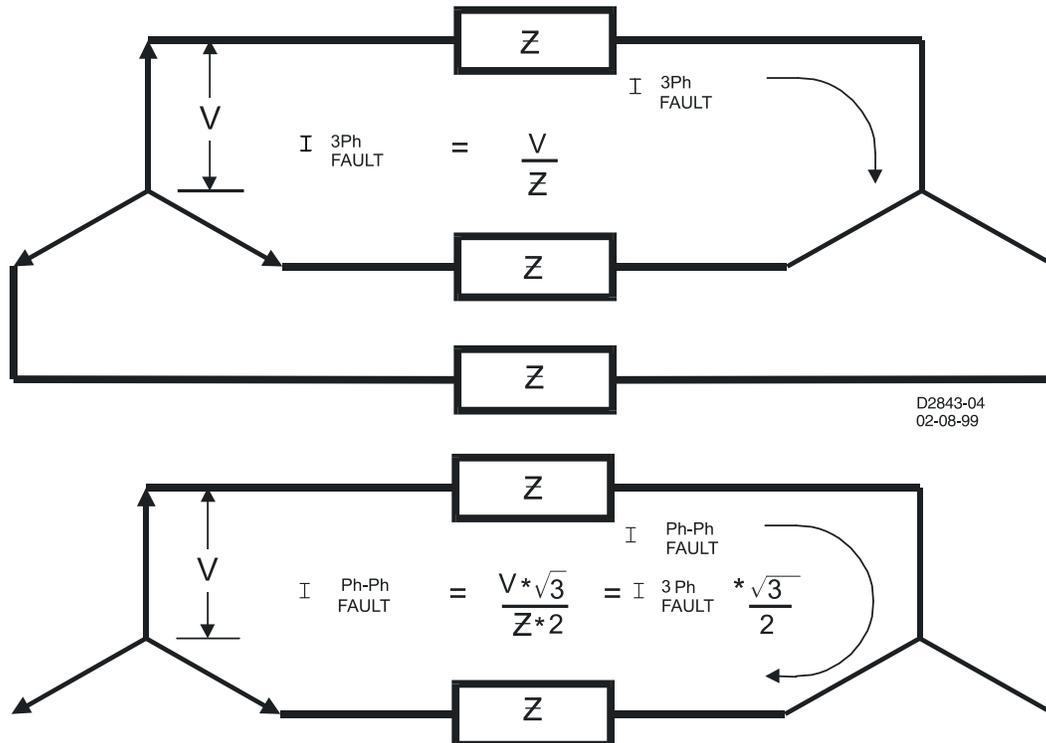
**Figure 24-1. Phase-to-Phase Fault Magnitude**
