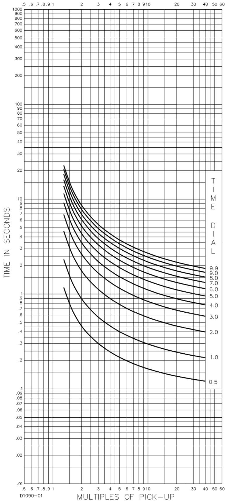
Figure 56-11. Time Characteristic Curve M, Moderately Inverse (Similar to ABB CO-7)
