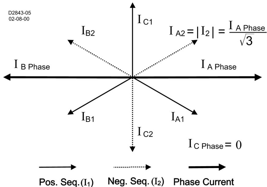
Figure 24-2. Sequence Components for an A-B Fault
