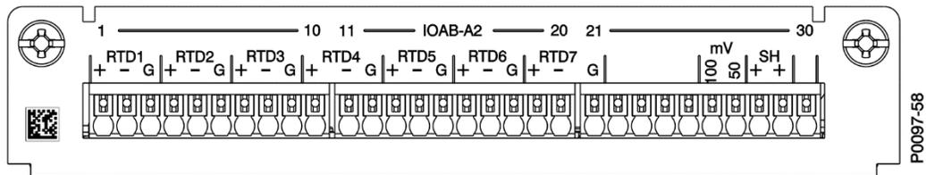
Figure 4-22. I/O and Auxiliary Board Connections, Option A2
