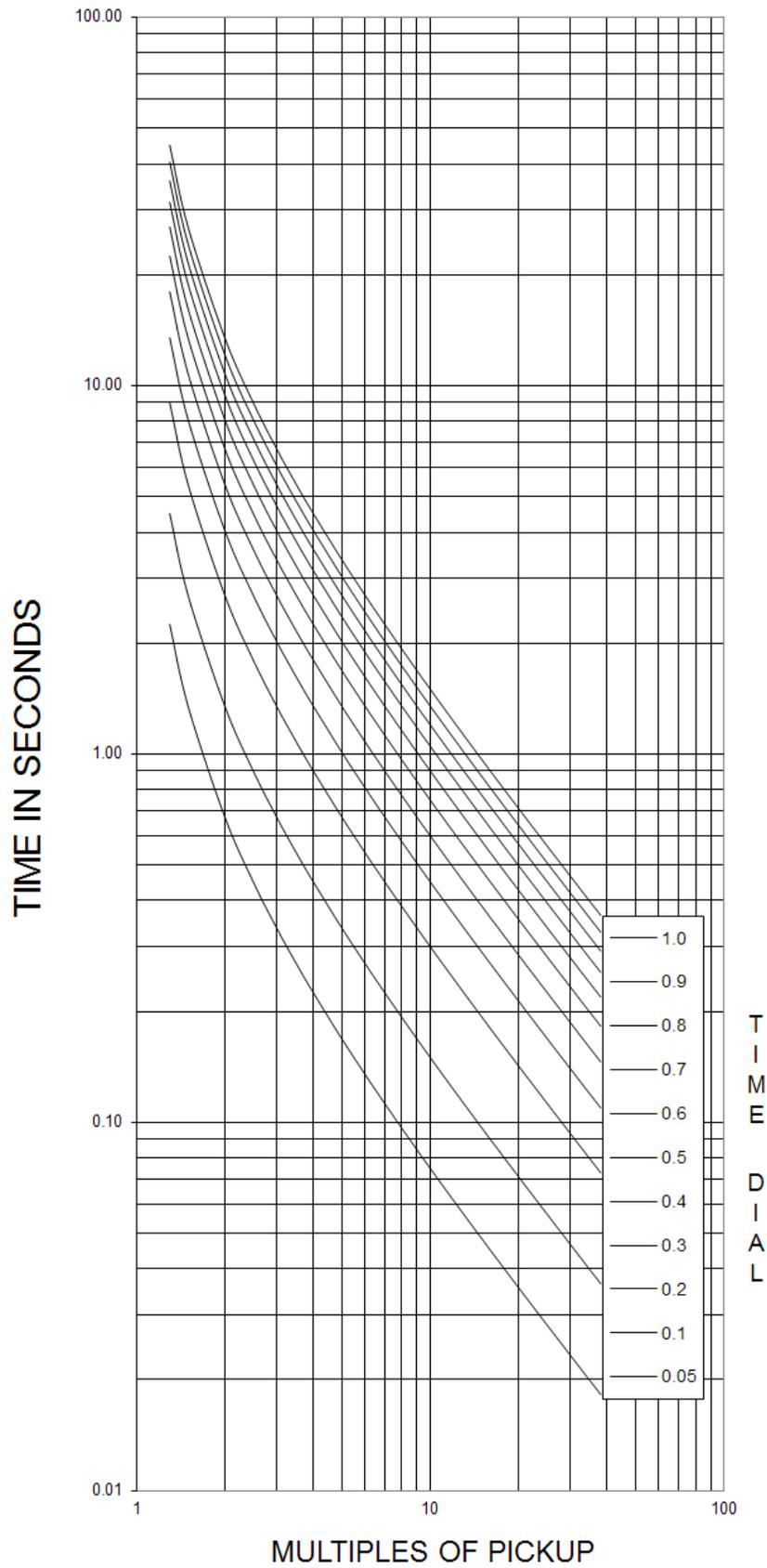
Figure 56-19. Time Characteristic Curve B1, Very Inverse (IEC 60255-151 Ed. 1)
