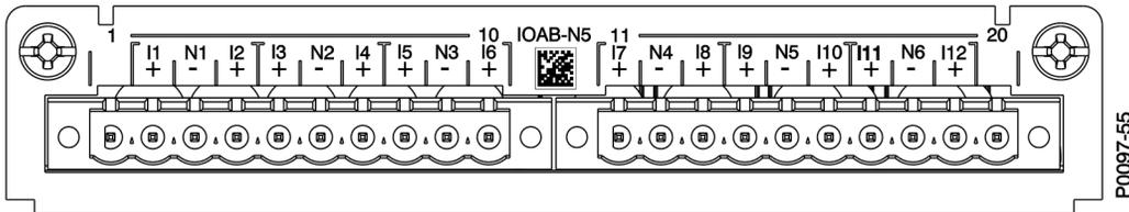
Figure 4-19. I/O and Auxiliary Board Connections, Option N5
