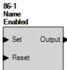
Figure 47-1. Virtual Lockout Function Element Logic Block
