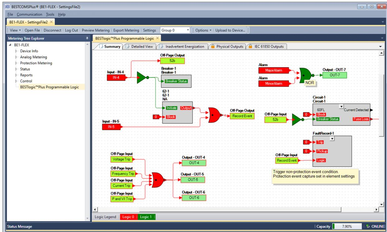
Figure 14-4. BESTlogic Plus Metering Screen
