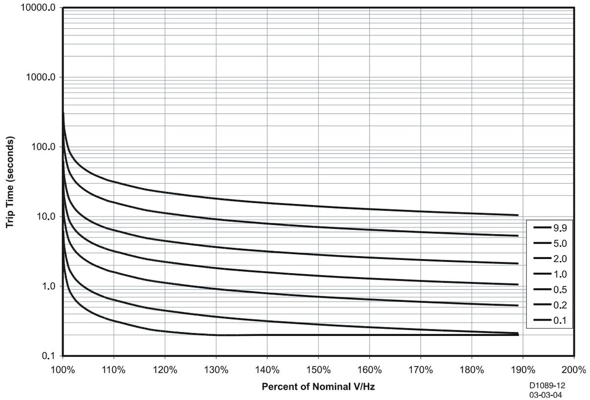
Figure 56-28. V/Hz Characteristic  $(M-1)^{0.5}$  – Time on Vertical Axis
