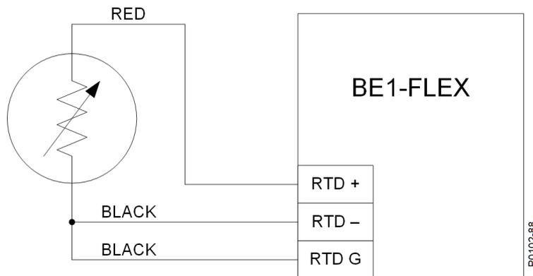
Figure 5-12. RTD Input – Three-Wire RTD Input Connections
