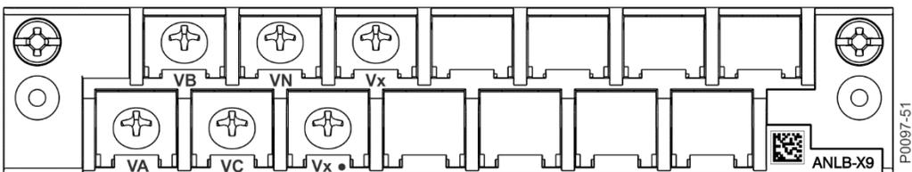
Figure 4-15. Analog Sensing Board Connections, Option X9
