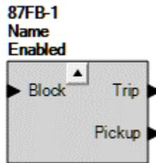
Figure 39-1. Flux Balance Element Logic Block
