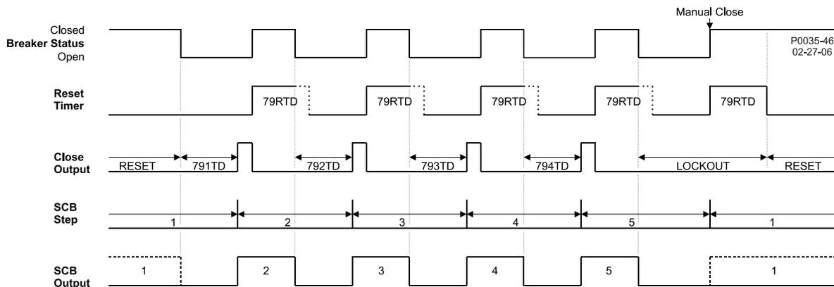
Figure 46-4. SCB=2/3/4/5 Logic Timing Diagram
