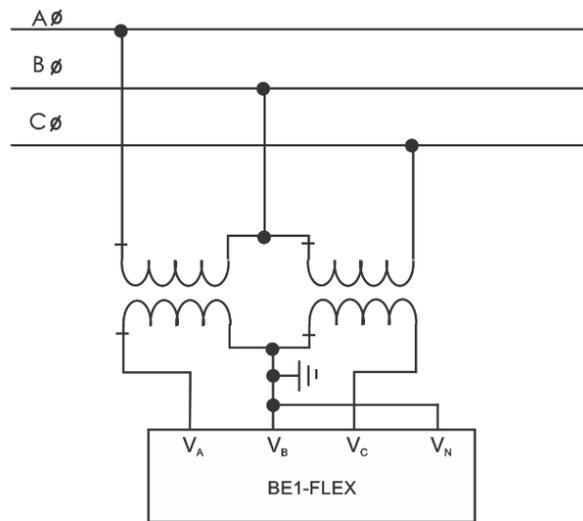
**B) Three Phase VTs; 3-Wire Connection**
