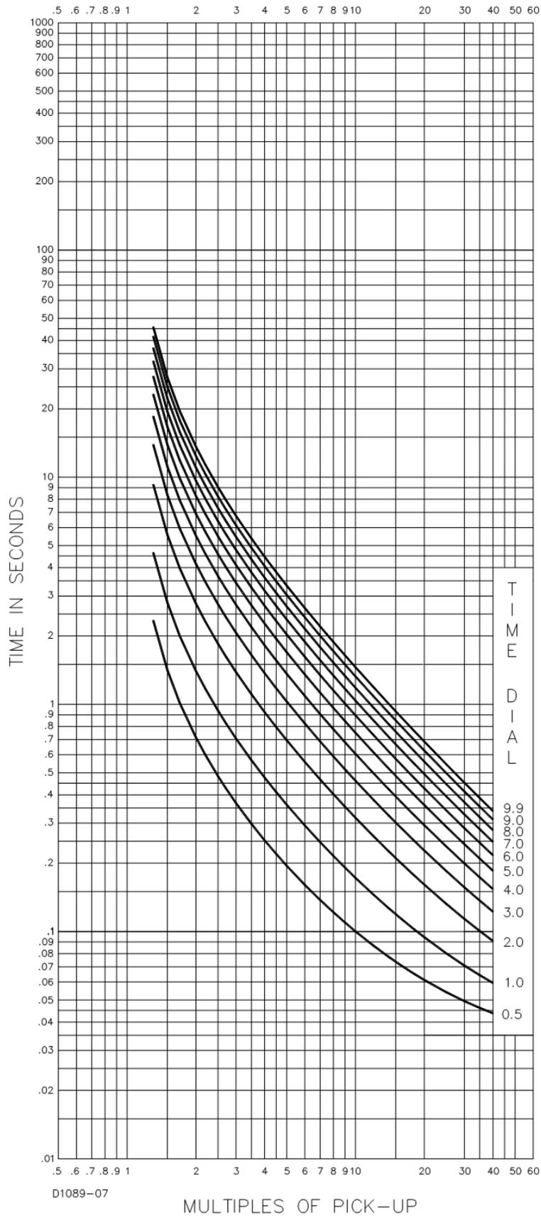
Figure 56-18. Time Characteristic Curve B, Very Inverse (BS 142)
