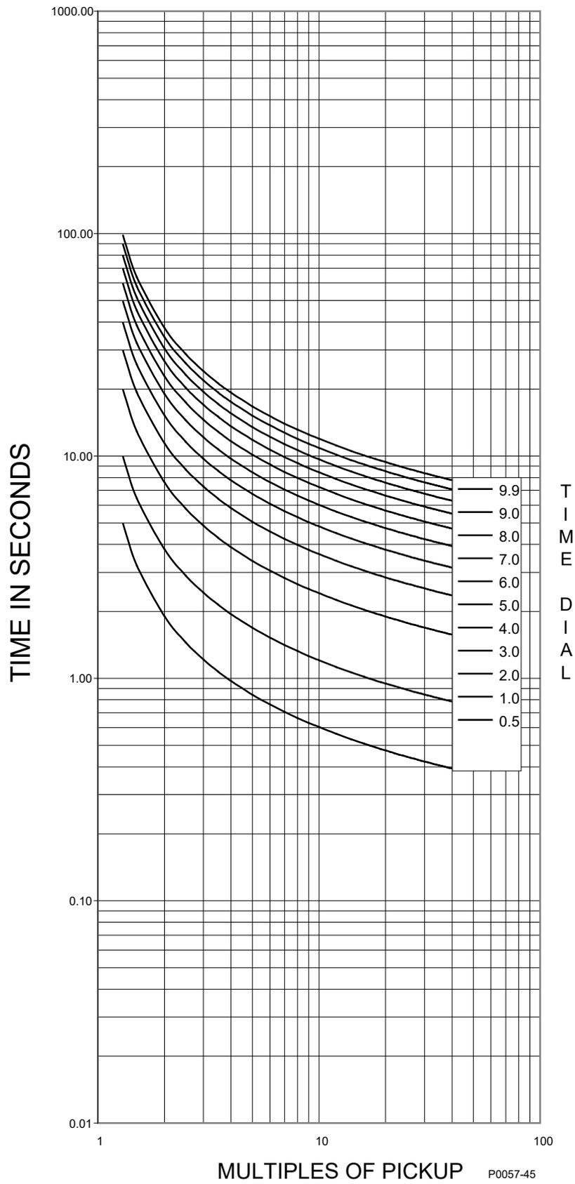
Figure 56-12. Time Characteristic Curve D1, Moderately Inverse (IEC 60255-151 Ed. 1)
