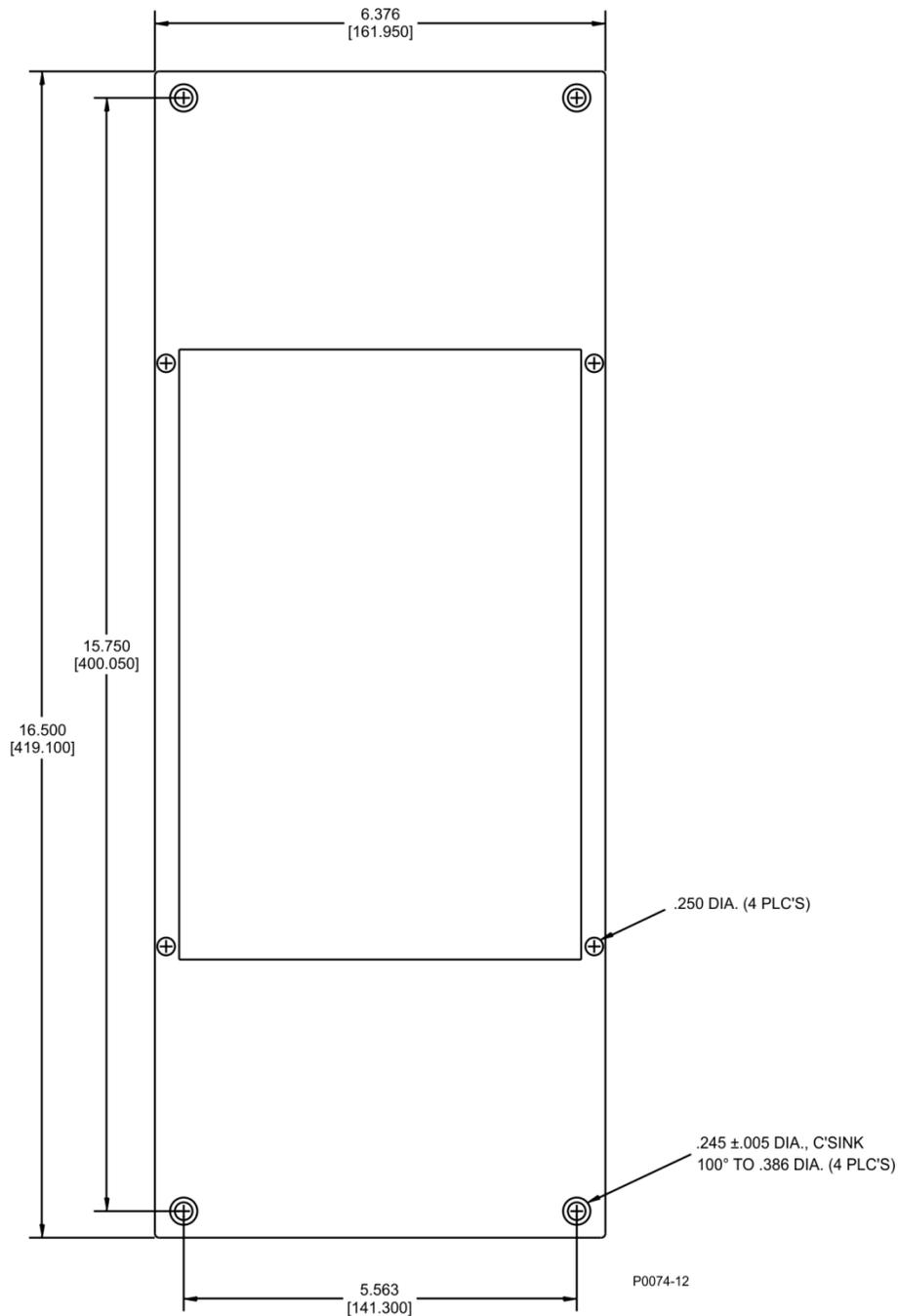
Figure 3-5. ABB FT-31/FT-32 Adapter Plate (Basler P/N: 9108551022)
