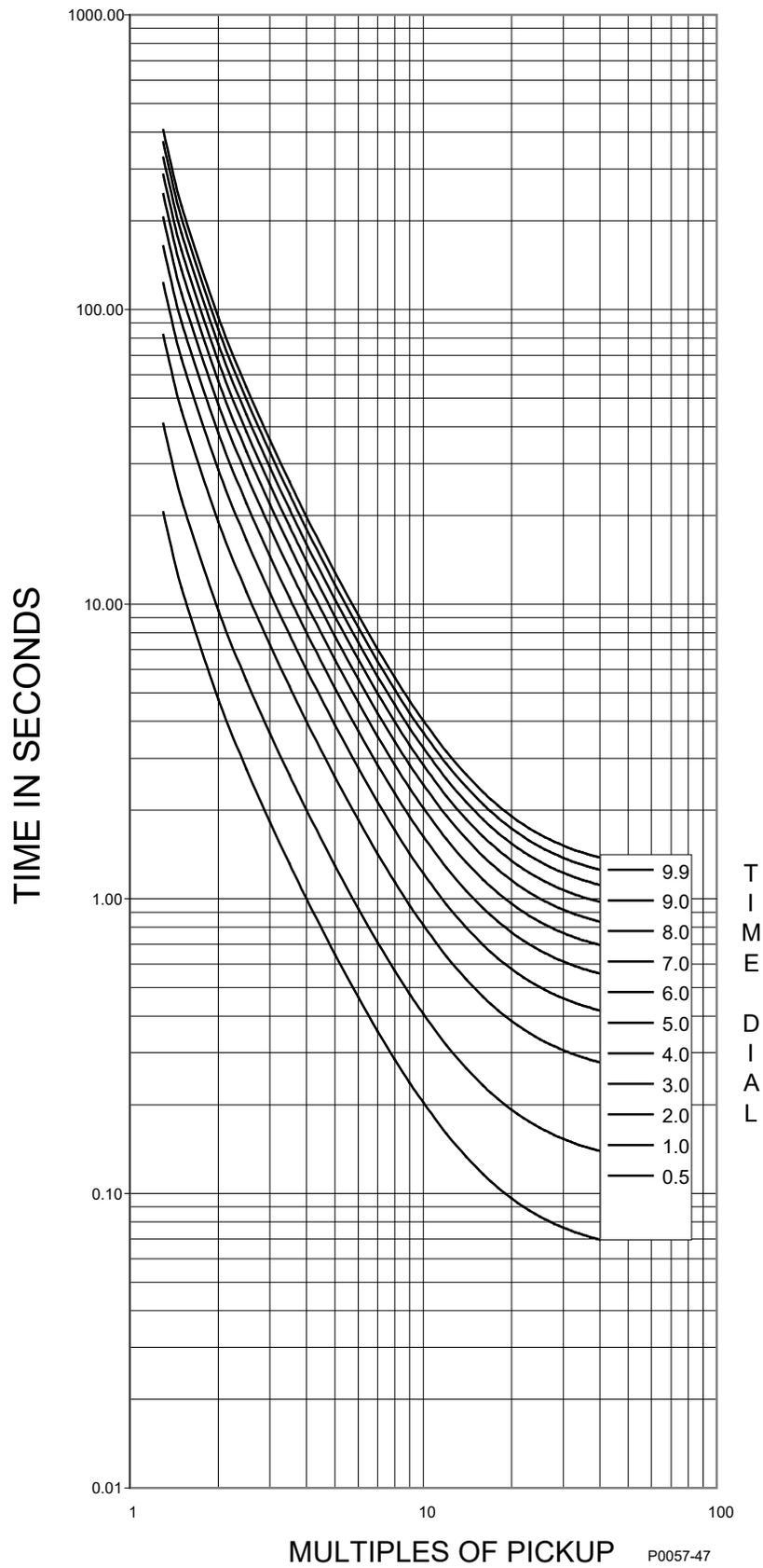
Figure 56-25. Time Characteristic Curve F1, Extremely Inverse (IEC 60255-151 Ed. 1)
