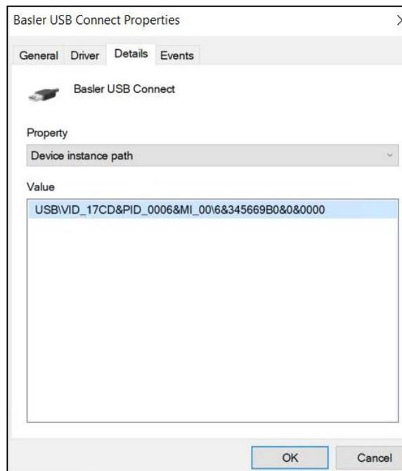
Figure 62-4. Basler USB Connect Properties
