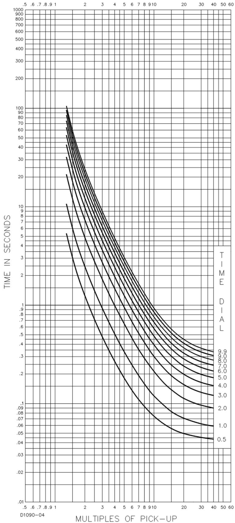
Figure 56-21. Time Characteristic Curve E1, Extremely Inverse (Similar to ABB CO-11)
