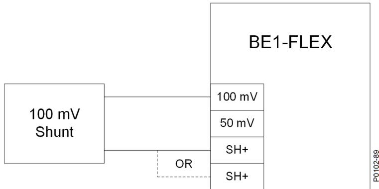
Note: If using a 50 mV shunt, connect wire to the 50 mV input.
