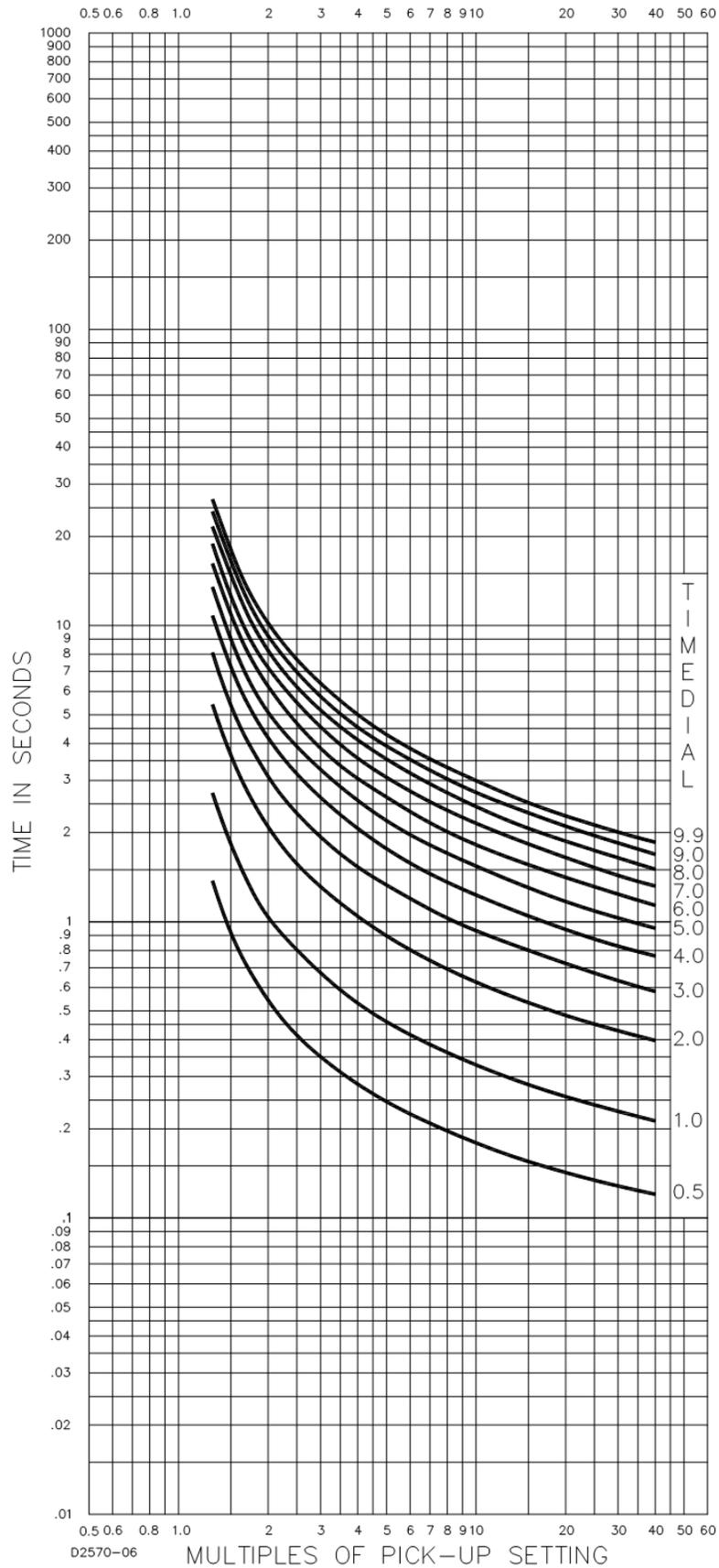
Figure 56-7. Time Characteristic Curve A, Standard Inverse (BS 142)
