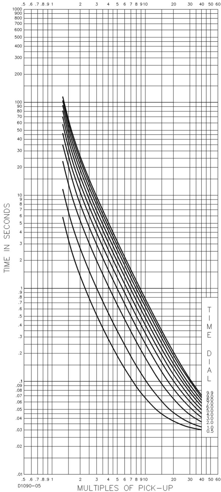
Figure 56-23. Time Characteristic Curve C, Extremely Inverse (BS 142)
