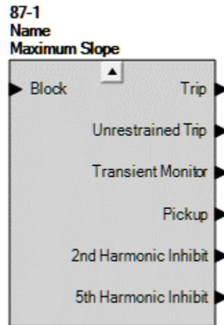
Figure 38-6. Phase Differential Element Logic Block
