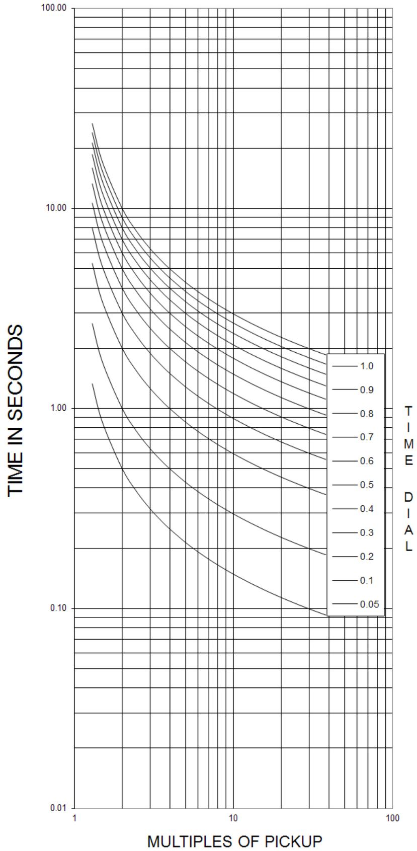
Figure 56-8. Time Characteristic Curve A1, Inverse (IEC 60255-151 Ed. 1)
