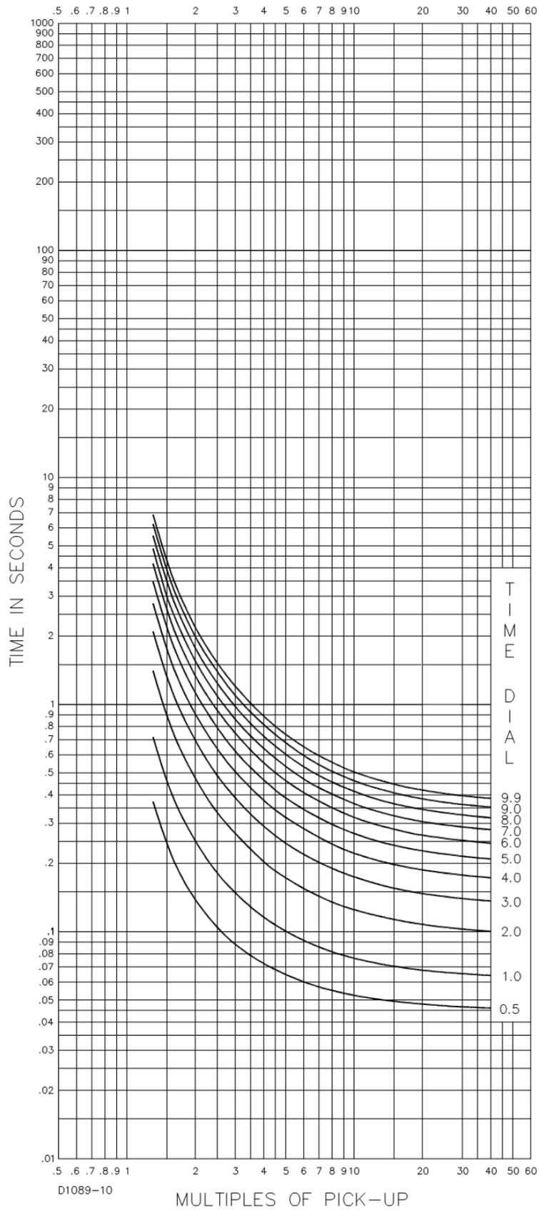
Figure 56-5. Time Characteristic Curve S1, Short Inverse (Similar to ABB CO-2)
