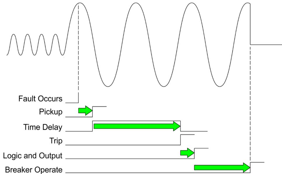
Figure 56-1. Element Operation Time
