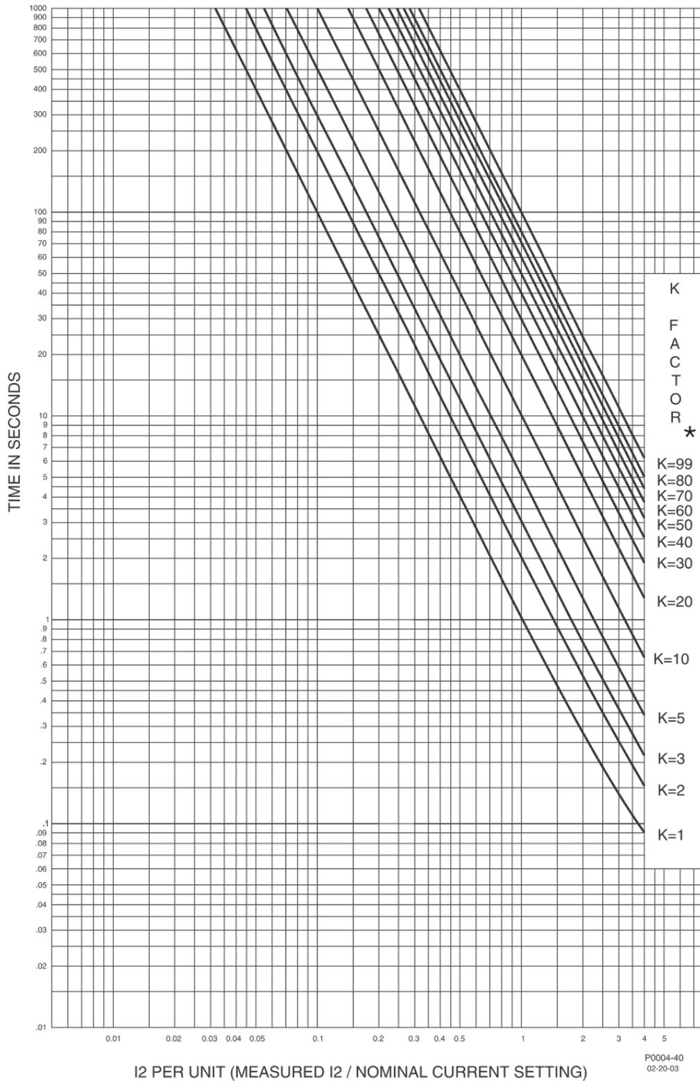
★ The K factor is the time that a generator can withstand 1 per-unit I2, where 1 pu is the user's setting for full-load current
