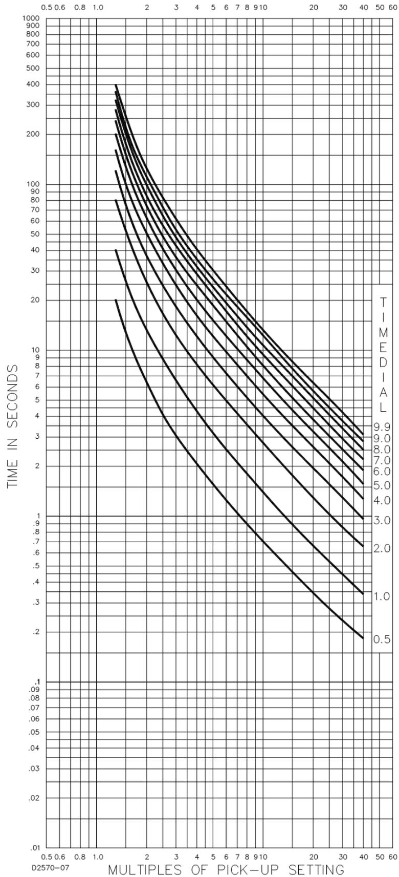
Figure 56-15. Time Characteristic Curve G, Long Time Inverse (BS 142)
