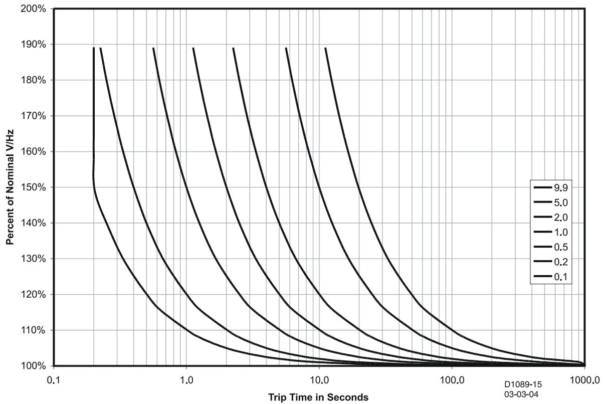
Figure 56-31. V/Hz Characteristic (M-1)<sup>1</sup> – Time on Horizontal Axis
