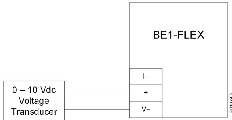
**Figure 5-9. Analog Input – Voltage Input Connections**
