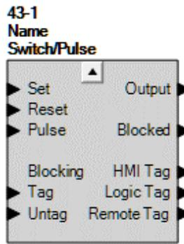
Figure 44-2. Virtual Control Switch Element Logic Block
