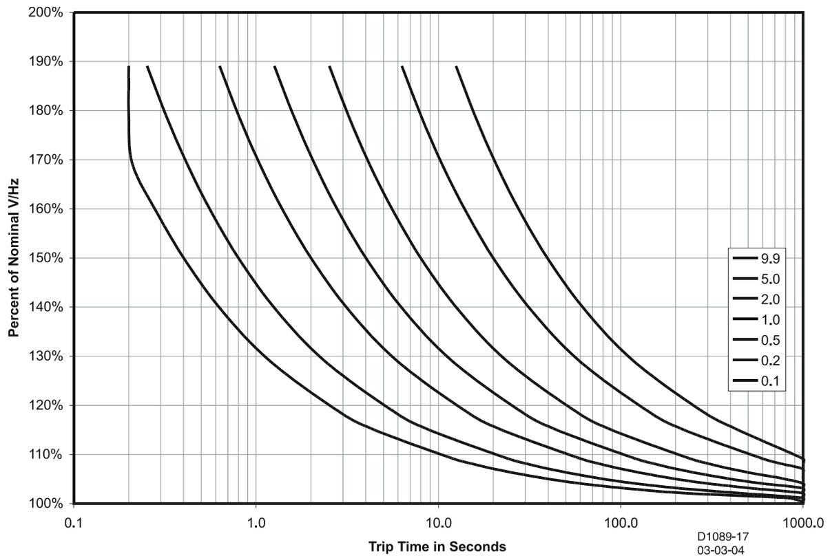
Figure 56-33. V/Hz Characteristic (M-1)<sup>2</sup> – Time on Horizontal Axis
