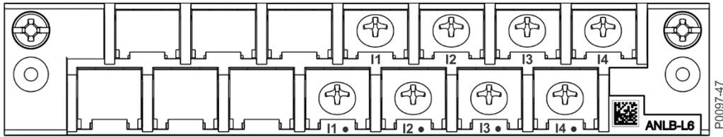
Figure 4-11. Analog Sensing Board Connections, Option L6
