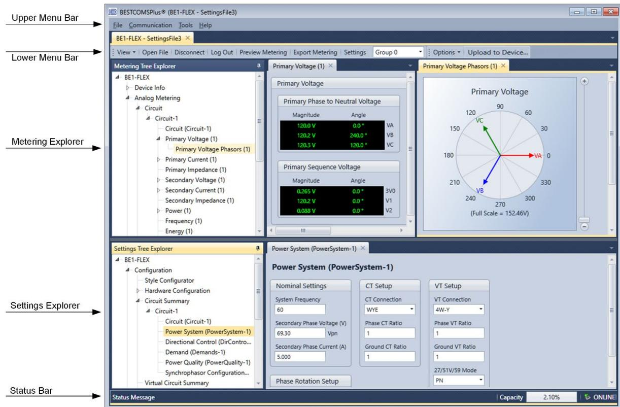
Figure 8-1. Typical User Interface Components
