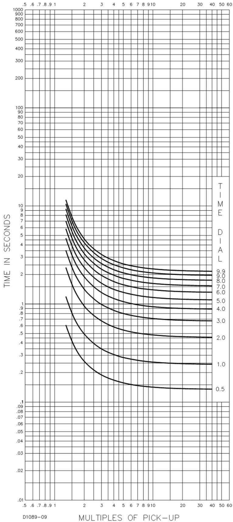
Figure 56-26. Time Characteristic Curve D, Definite Time (Similar To ABB CO-6)
