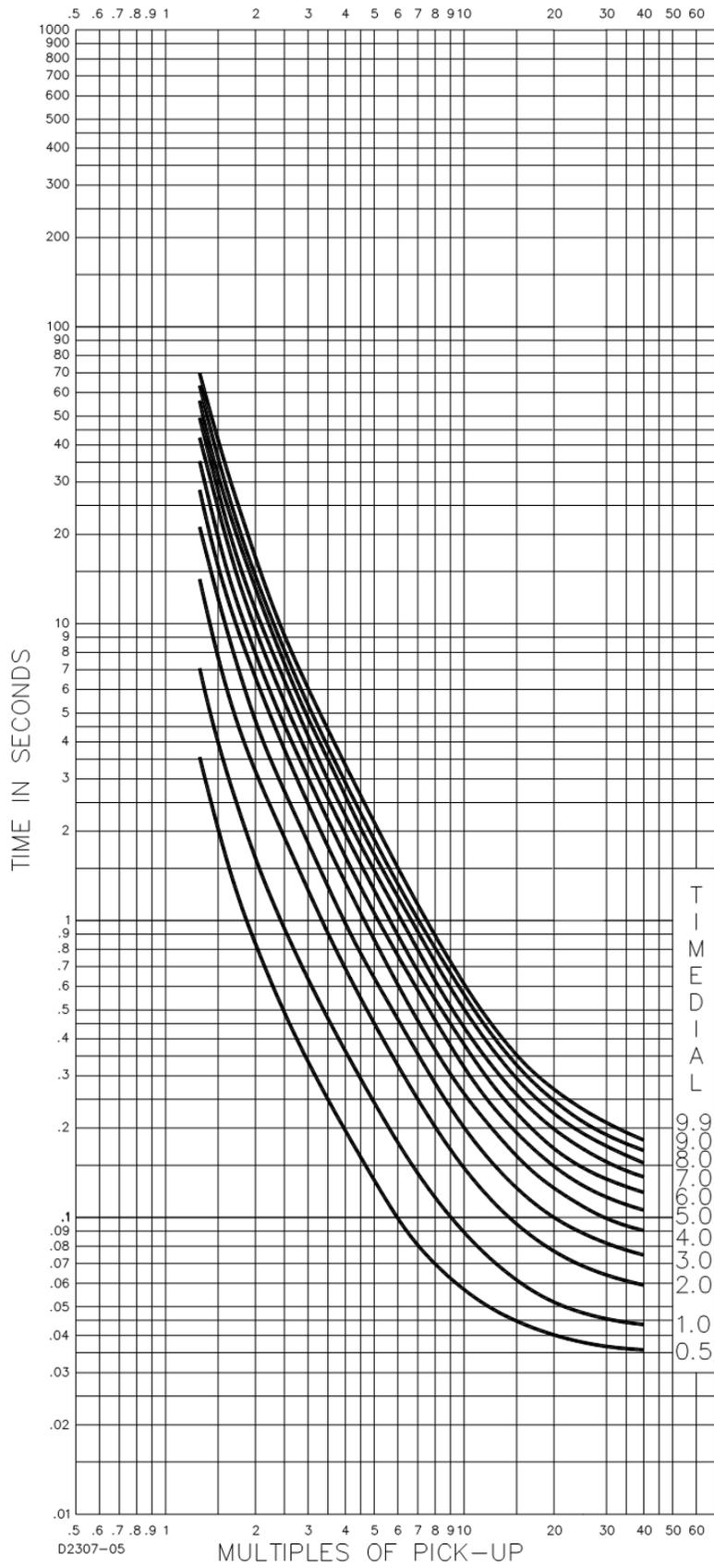
Figure 56-22. Time Characteristic Curve E2, Extremely Inverse (Similar to GE IAC-77)
