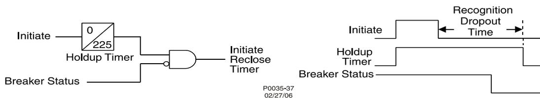
**Figure 46-1. Recognition Dropout Timing**
