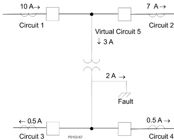
**Figure 38-5. Virtual Circuit 5 Example**
