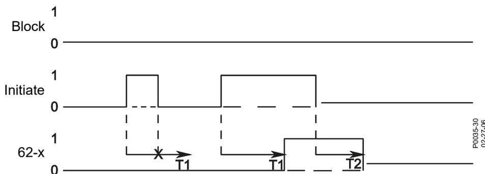
Figure 45-1. Pickup/Dropout Mode
