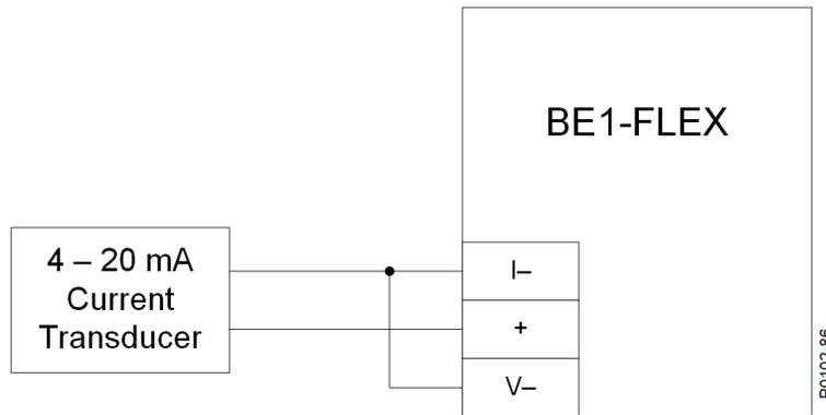
Figure 5-10. Analog Input – Current Input Connections
