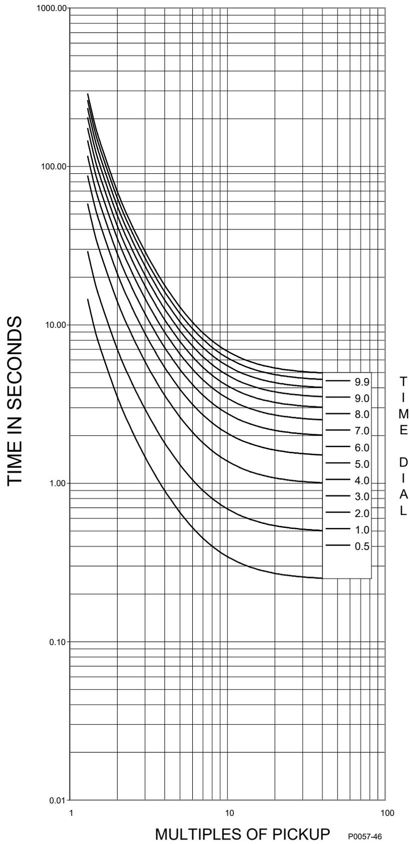
Figure 56-20. Time Characteristic Curve E3, Very Inverse (IEC 60255-151 Ed. 1)
