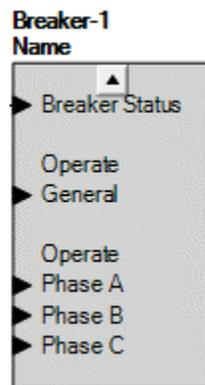
Figure 10-22. Breaker Status Logic Block
