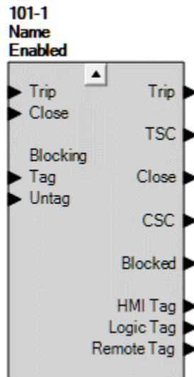
Figure 48-3. Breaker Control Element Logic Block
