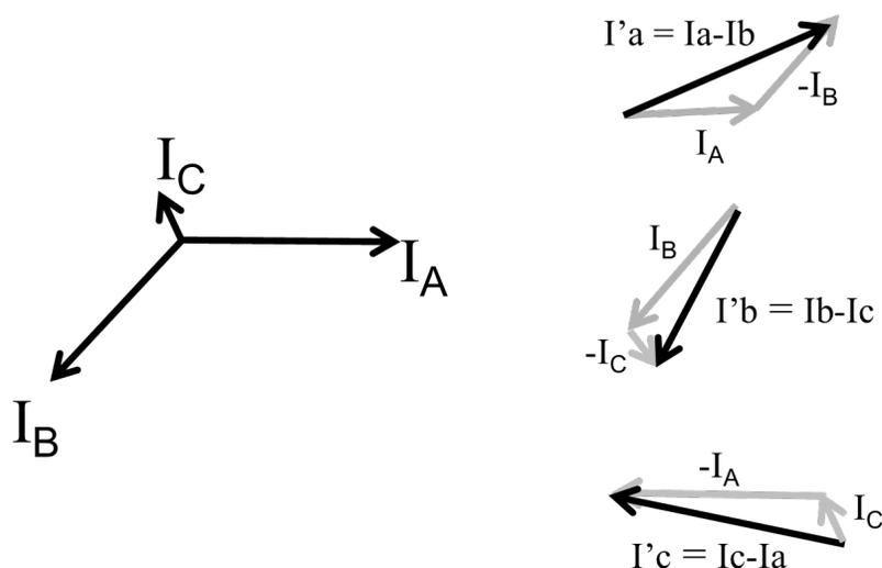
**Figure 38-9. Phasor measurements with DAB compensated currents**
