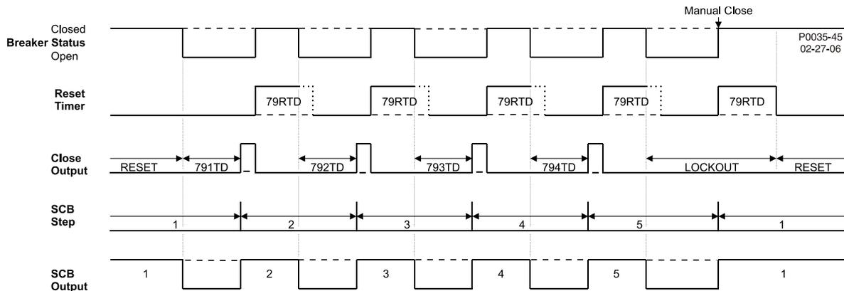
Figure 46-3. SCB=1/2/3/4/5 Logic Timing Diagram
