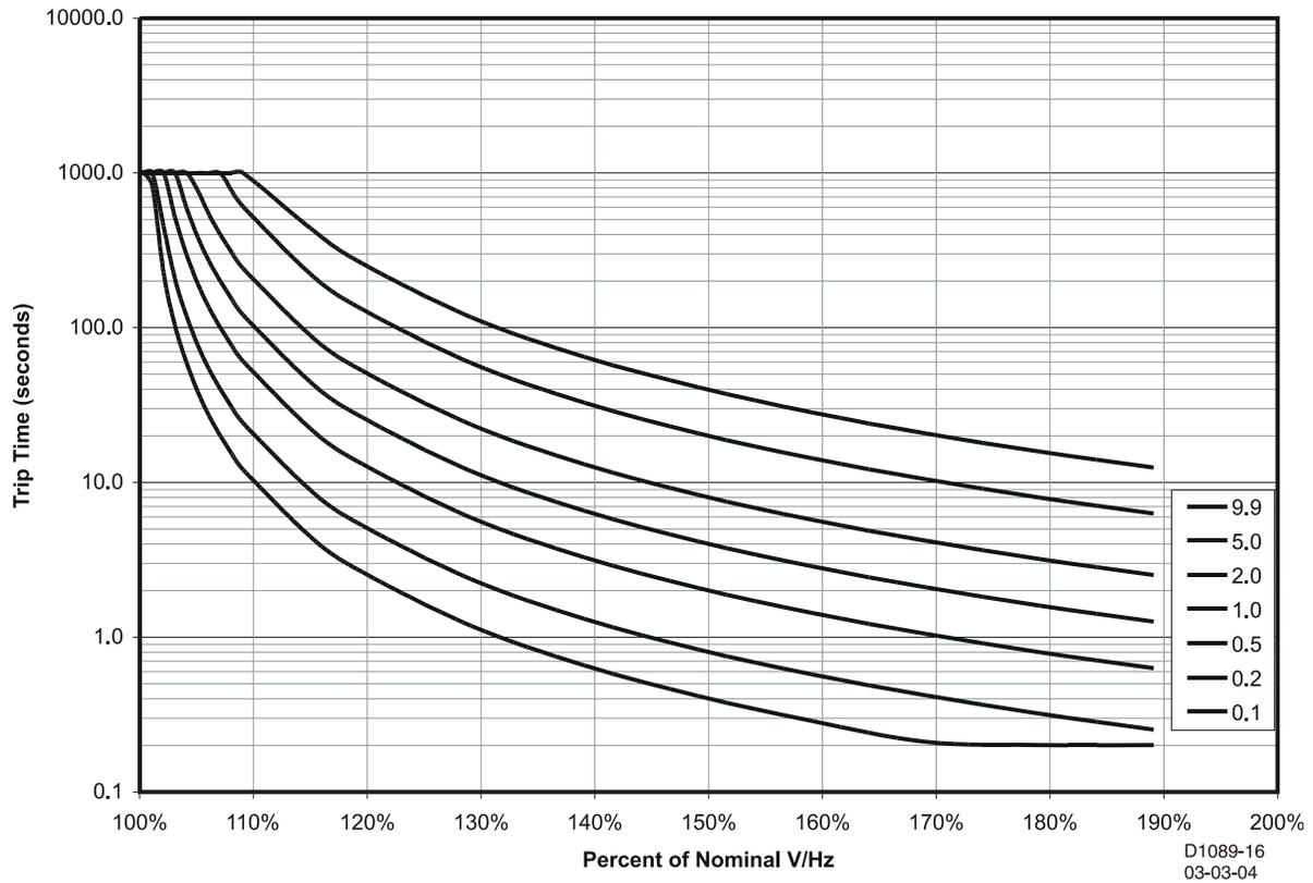
Figure 56-32. V/Hz Characteristic (M-1)<sup>2</sup> – Time on Vertical Axis
