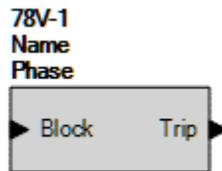
Figure 36-2. Vector Jump Element Logic Block
