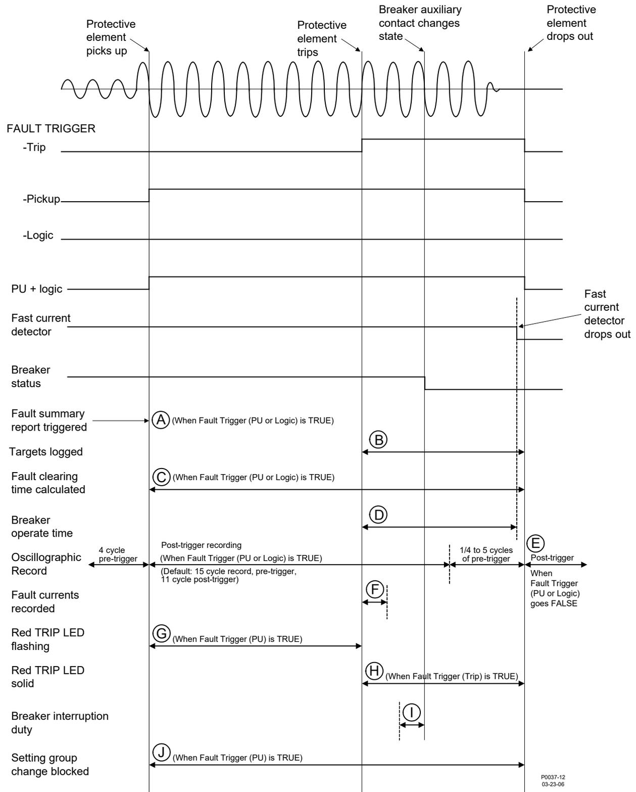
Figure 53-9. Protective Fault Analysis
