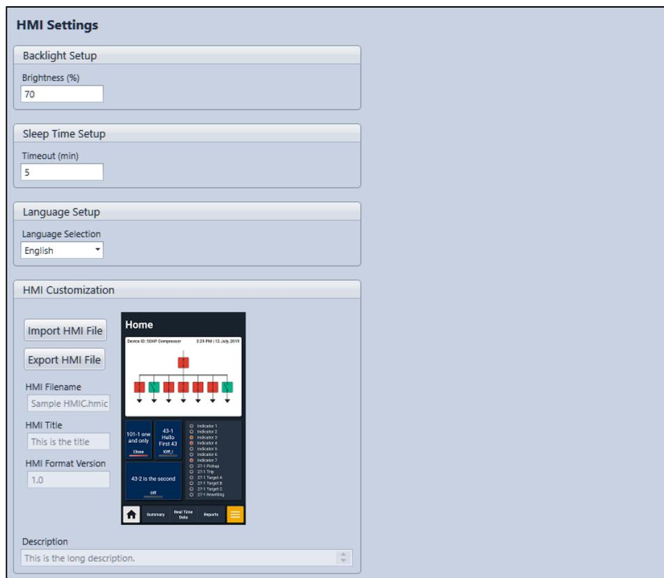
Figure 7-5. HMI Settings Screen
