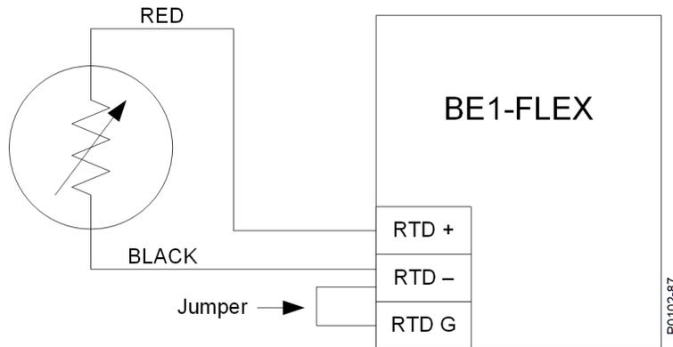
Figure 5-11. RTD Input – Two-Wire RTD Input Connections
