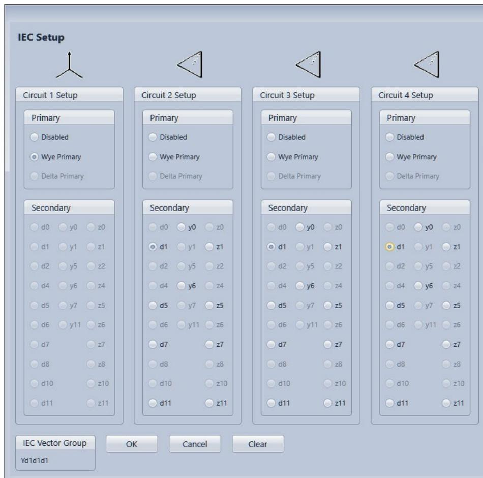
Figure 38-4. IEC Transformer Setup Screen
