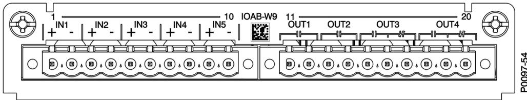
Figure 4-18. I/O and Auxiliary Board Connections, Option W9
