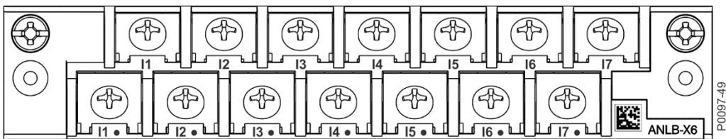
Figure 4-13. Analog Sensing Board Connections, Option X6
