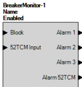
**Figure 10-21. Breaker Monitor Logic Block**
