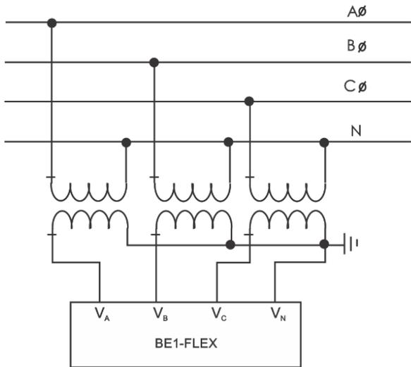
**A) Three Phase VTs; 4-Wire Connection**
