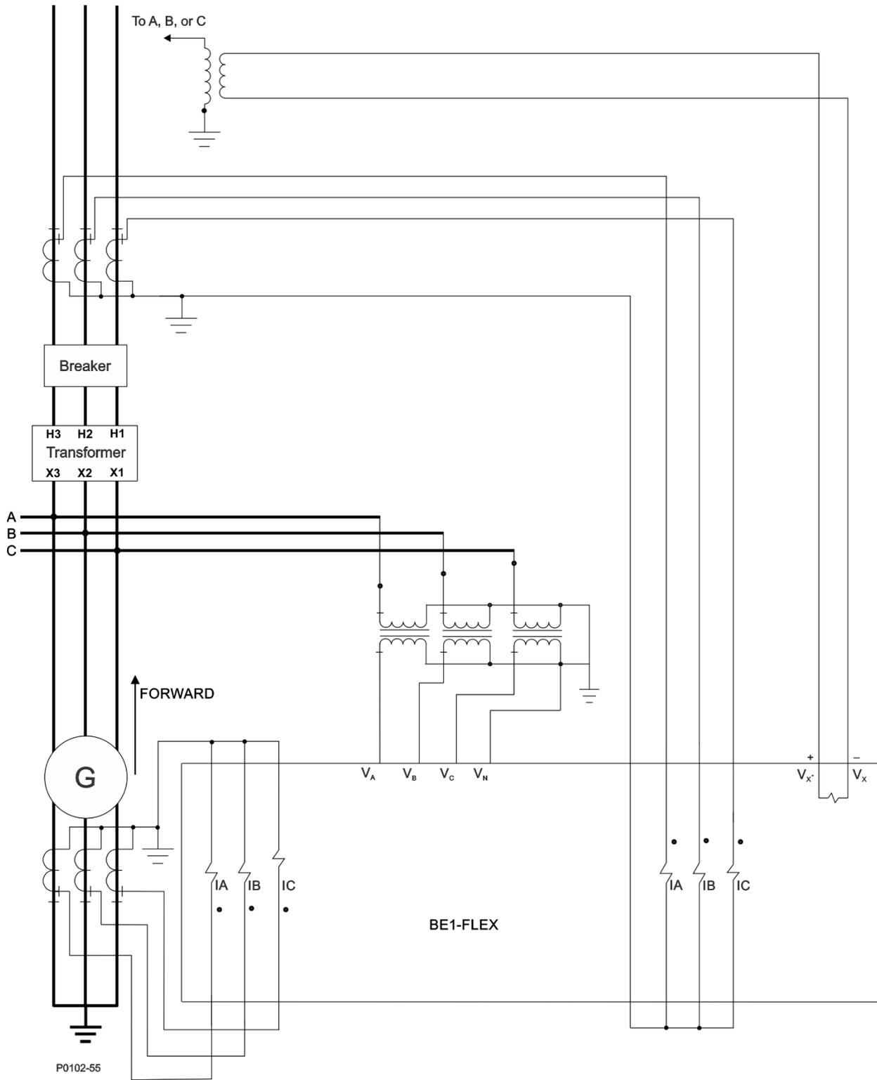
Figure 5-4. Typical AC Connections for Overall Differential
