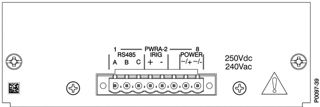
Figure 4-3. Power Supply Board Connections, Option 2
