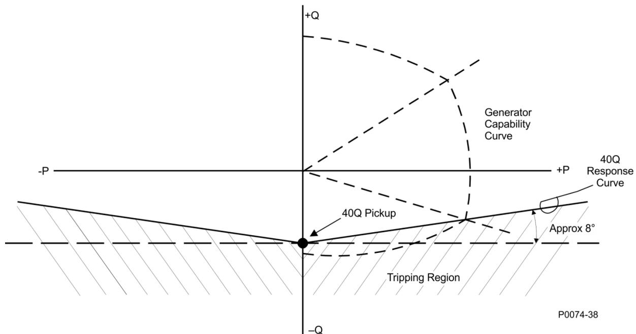
Figure 22-1. Generator Capability Curve vs. 40Q Response
