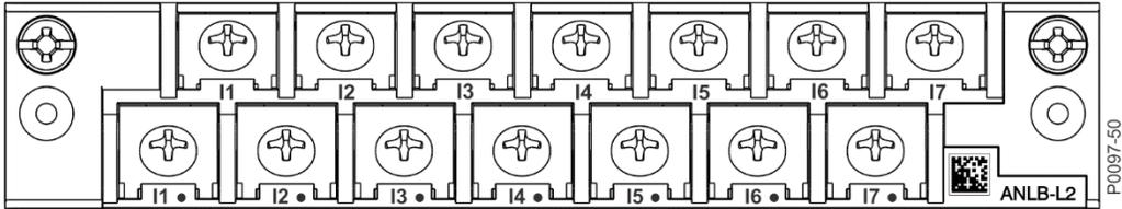
Figure 4-14. Analog Sensing Board Connections, I7 = SEF Channel, Option L2
