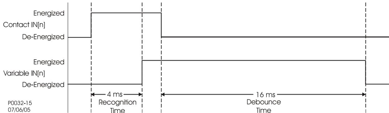
Figure 10-25. Digital Input Conditioning Timing Diagram
