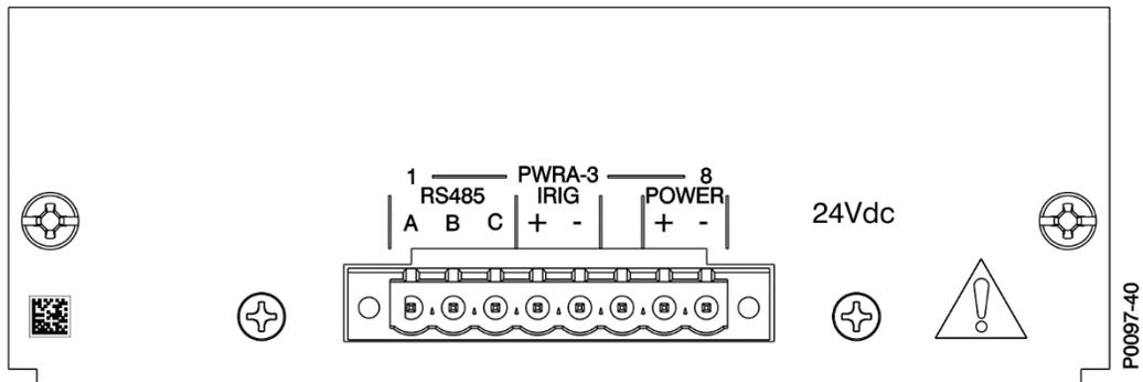
Figure 4-4. Power Supply Board Connections, Option 3
