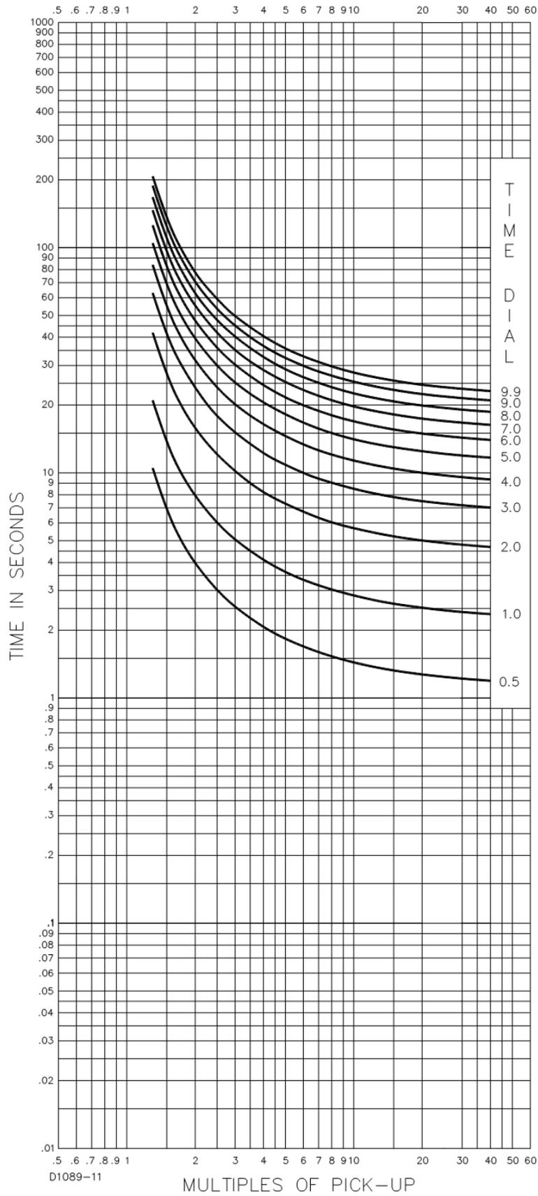
Figure 56-13. Time Characteristic Curve L1, Long Inverse (Similar to ABB CO-5)
