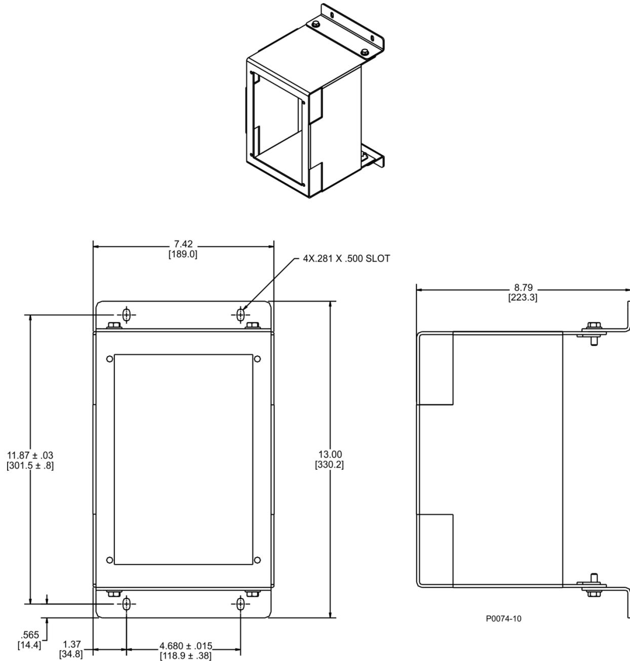
Figure 3-9. Pivoting Projection-Mounting Kit (Basler P/N: 9424226101)
