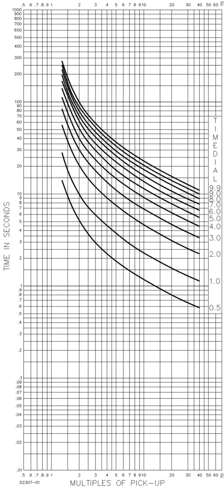
Figure 56-14. Time Characteristic Curve L2, Long Inverse (Similar To GE IAC-66)
