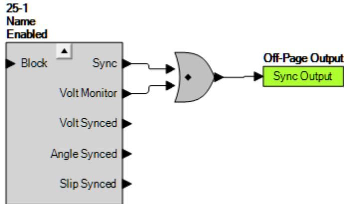
Figure 18-2. Sync-Check Element Logic Block
