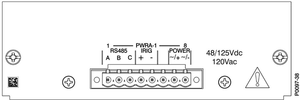
Figure 4-2. Power Supply Board Connections, Option 1
