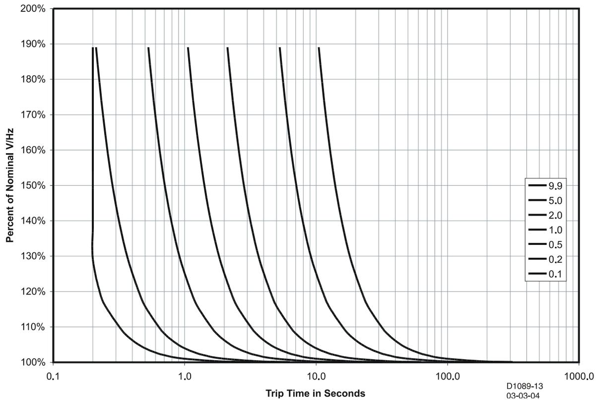
Figure 56-29. V/Hz Characteristic  $(M-1)^{0.5}$  – Time on Horizontal Axis
