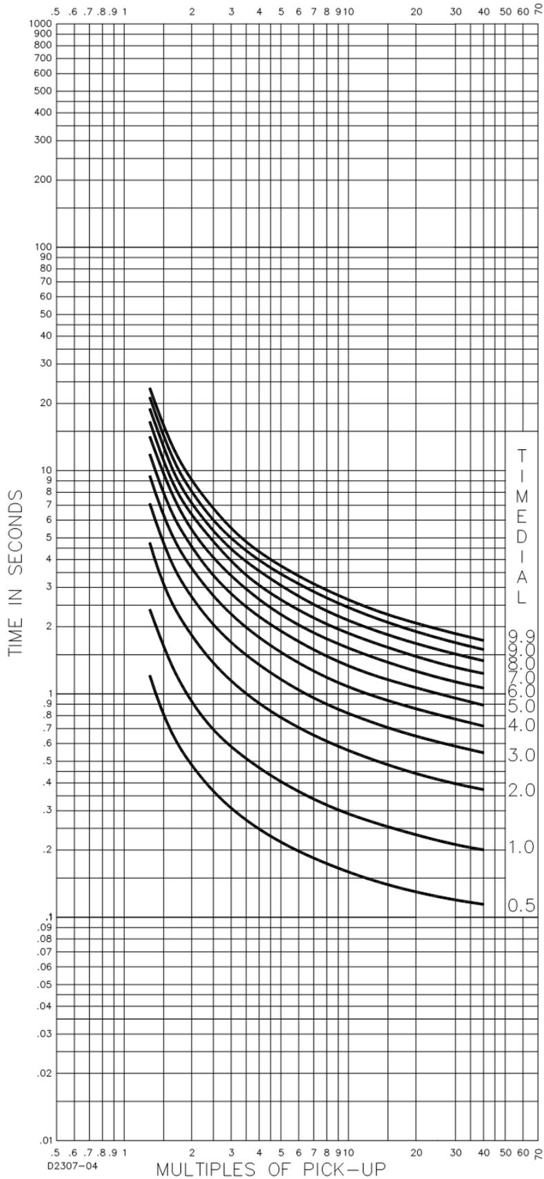
Figure 56-10. Time Characteristic Curve I2, Inverse Time (Similar to GE IAC-51)
