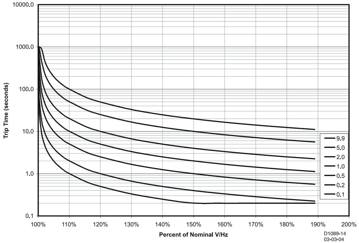
Figure 56-30. V/Hz Characteristic (M-1)<sup>1</sup> – Time on Vertical Axis
