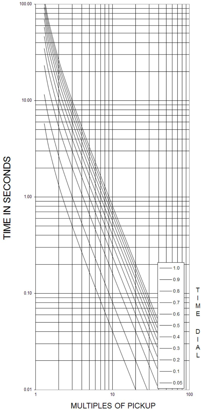
Figure 56-24. Time Characteristic Curve C1, Extremely Inverse (IEC 60255-151 Ed. 1)
