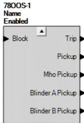
Figure 35-2. Out of Step Element Logic Block
