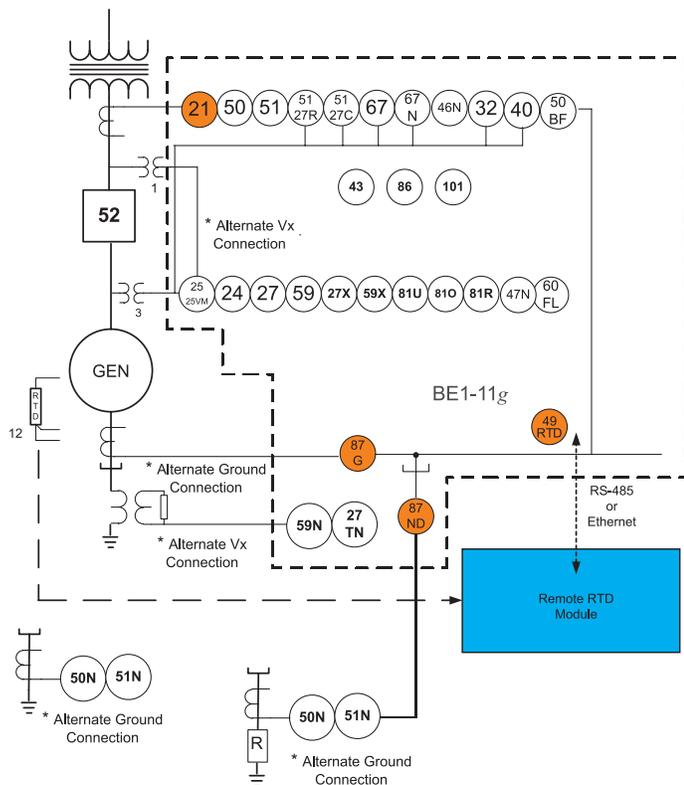
Figure 7 - BEI-11g Generator Application
