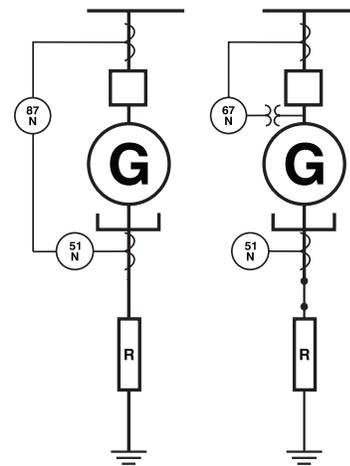
**Figure 4 - Stator Ground Fault Protection in Low-Impedance Grounded Generators**
