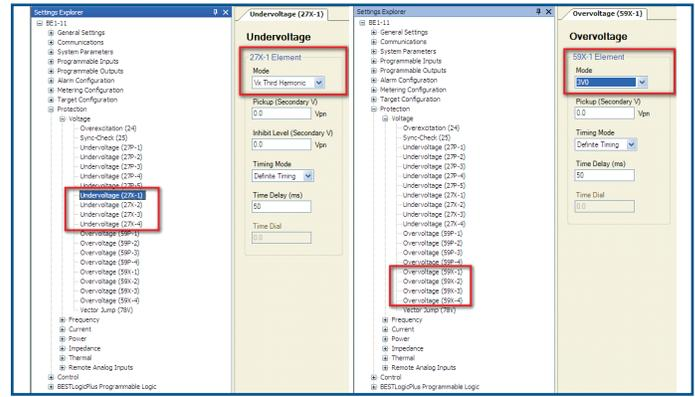
Figure 6 - Voltage Elements in BESTCOMSPPlus
