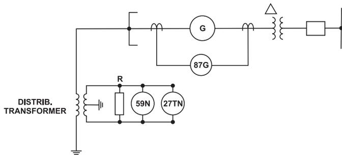
**Figure 2 - Stator Phase and Ground Fault Protection in High-Impedance Grounded Generators**
