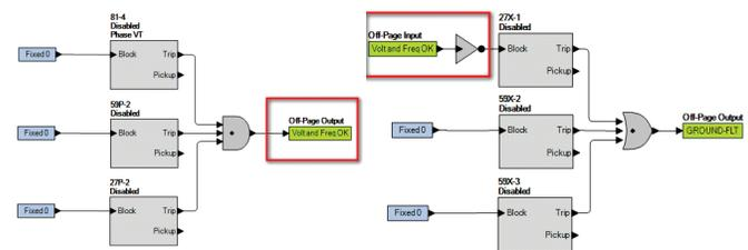
**Figure 3 - The Use of 27/59 and 81 Elements to Supervise 27TN in BESTlogic™ Plus**
