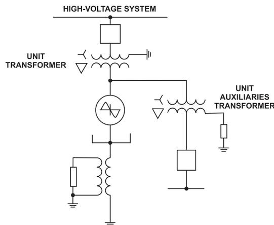
Figure 1 - Unit Generator-Transformer Configuration with Generator Breaker on High Side of a Transformer. (Reference IEEE Std. C37.102 – 2006)
