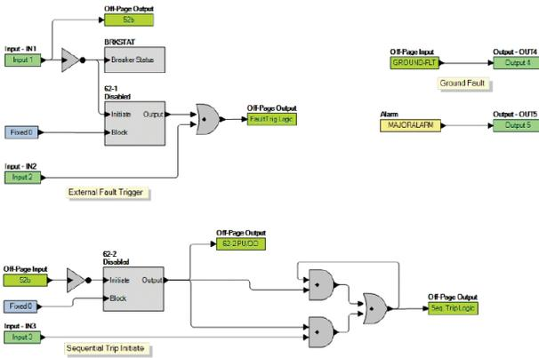
Figure 9 - A Sample of High-Impedance Grounded Generator Protection Logic in BESTspace
