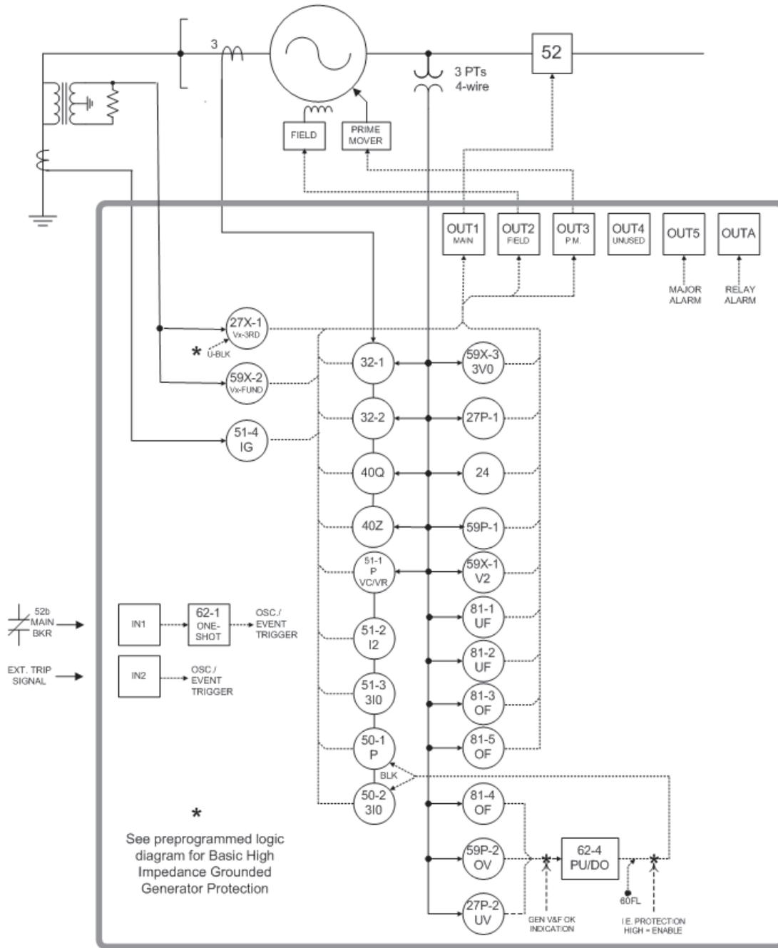
Figure 8 - Expanded version of Figure 1: One-Line Diagram of Basic High Impedance Generator Protection
