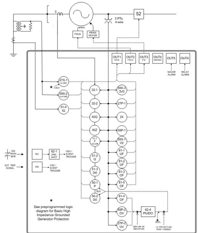
Figure 1 - One-Line Diagram of Basic High Impedance Generator Protection
