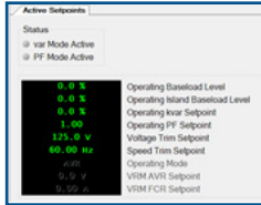
Figure 29d - Active Setpoints Metering
