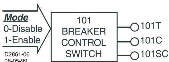
Figure 4-42. Virtual Breaker Control Switch Logic Block
