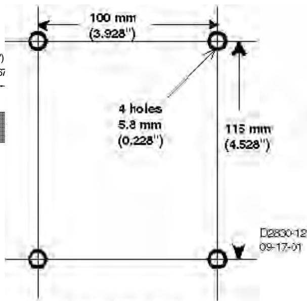
Figure 4. Drilling Template
