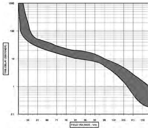
Figure 2. Typical Inverse Time Delay Characteristic Curve
