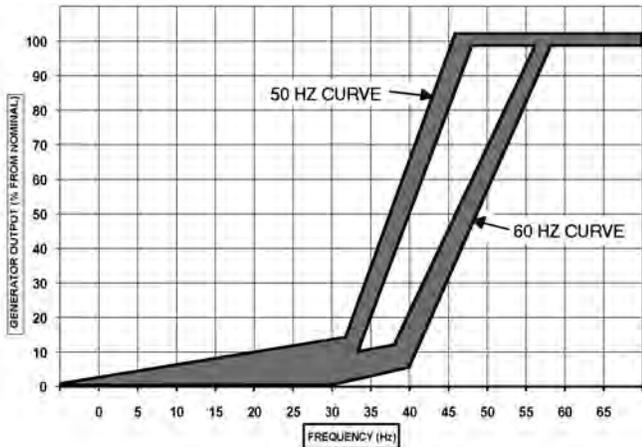
Figure 1. Frequency Compensation Curves
