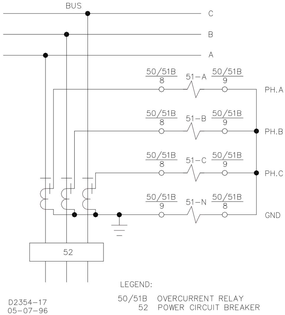
**Figure 4-2. AC Input Connections**
