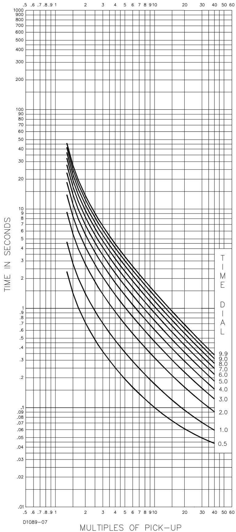
Figure 7-8. Time Characteristic Curve, BS142-B (BS142 Very Inverse)
