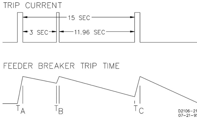
**Figure 4-1. Coordination Timing Diagram**
