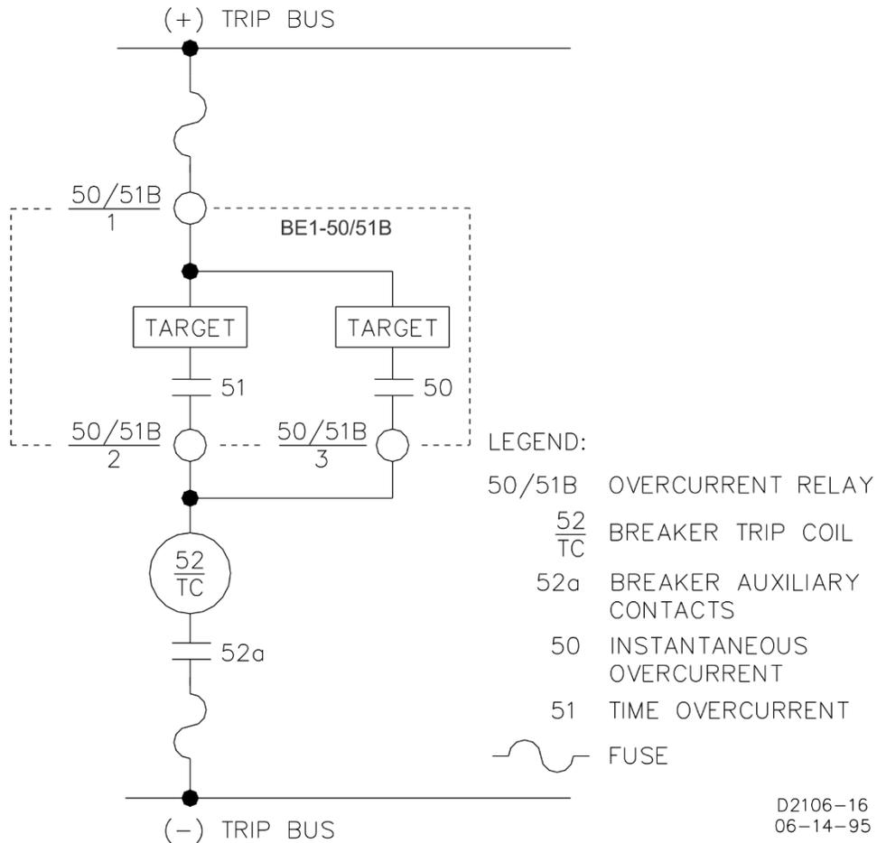
**Figure 4-3. DC Control Connections, BE1-50/51B-214/-225**
