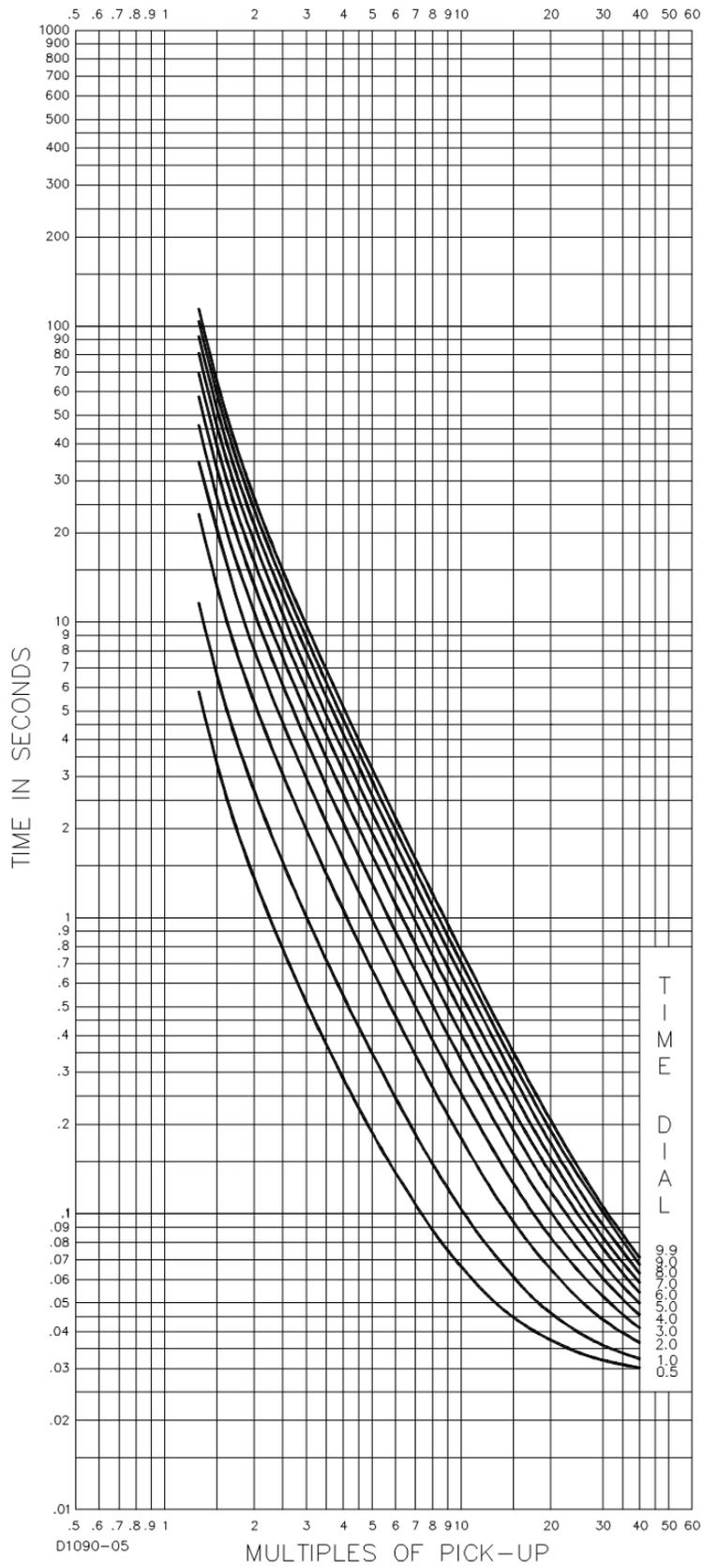
Figure 7-9. Time Characteristic Curve, BS142-C (BS142 Extremely Inverse)
