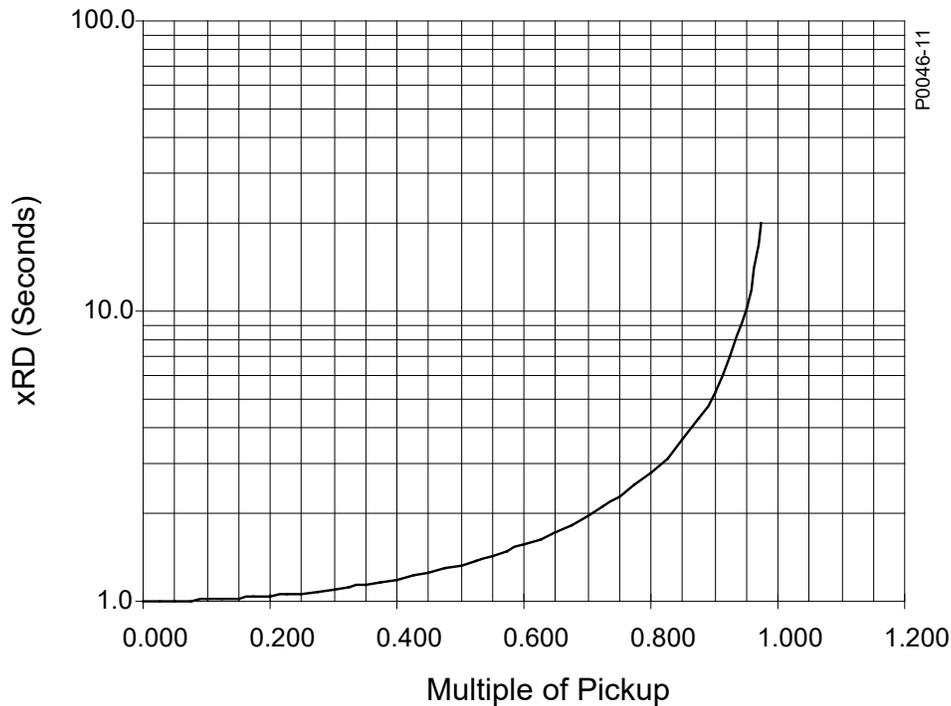
Vertical axis xRD (Seconds) is applicable for all curves and is derived from multiplying the constant R for the curve selected times D (the Time Dial setting).
