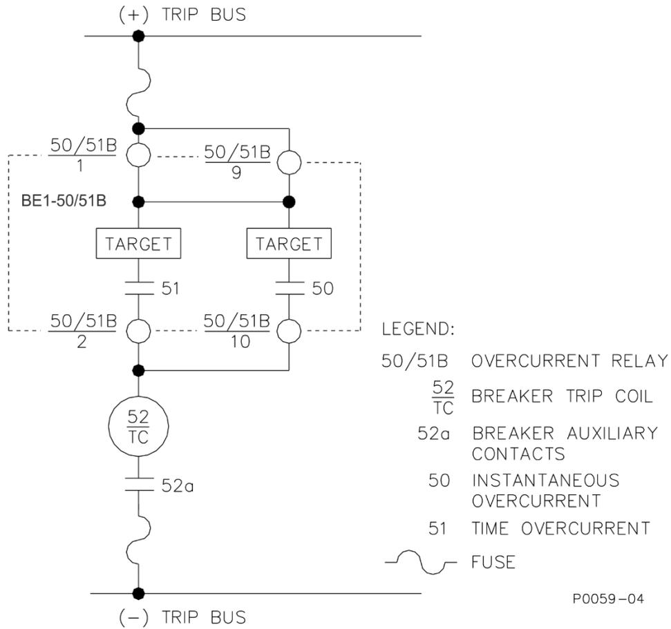
Figure 4-4. DC Control Connections, BE1-50/51B-215
