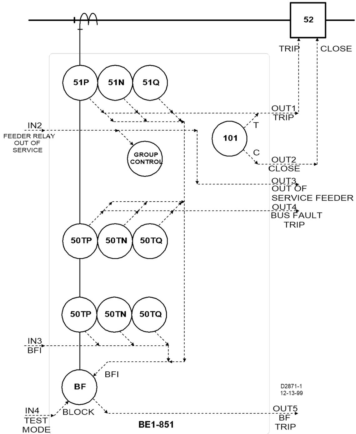
Figure 8-13. Typical One-Line Diagram for Backup Logic
