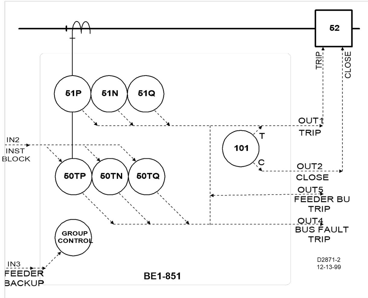
Figure 8-11. Typical One-Line Diagram for BUS Logic
