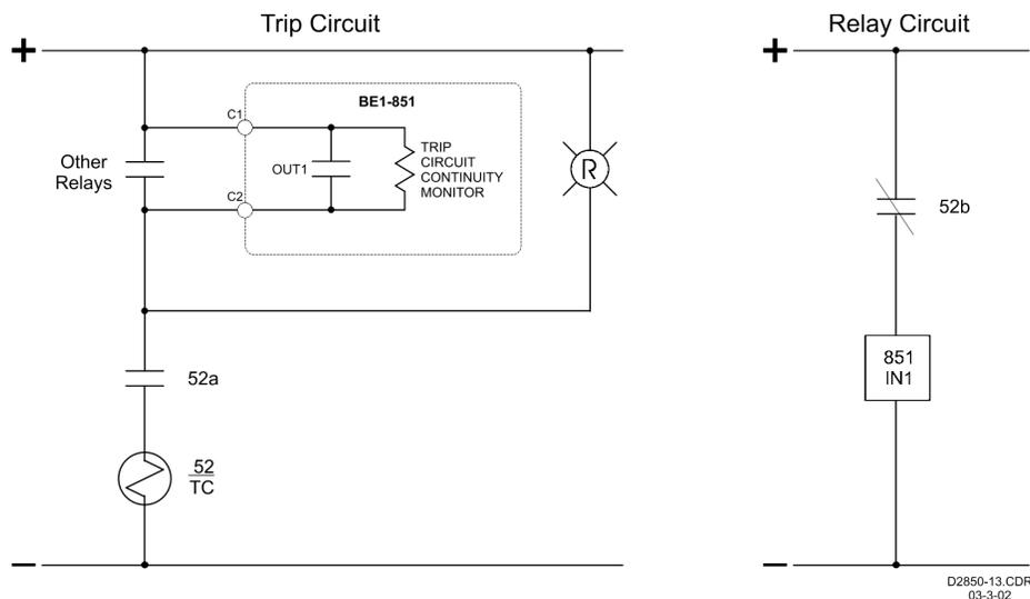
Figure 6-10. Trip Circuit Voltage and Continuity Monitor
