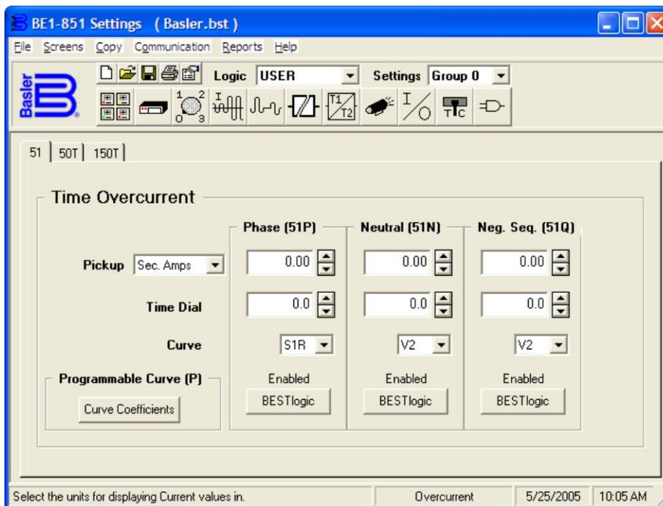
Figure 14-10. Time Overcurrent Screen, 51 Tab
