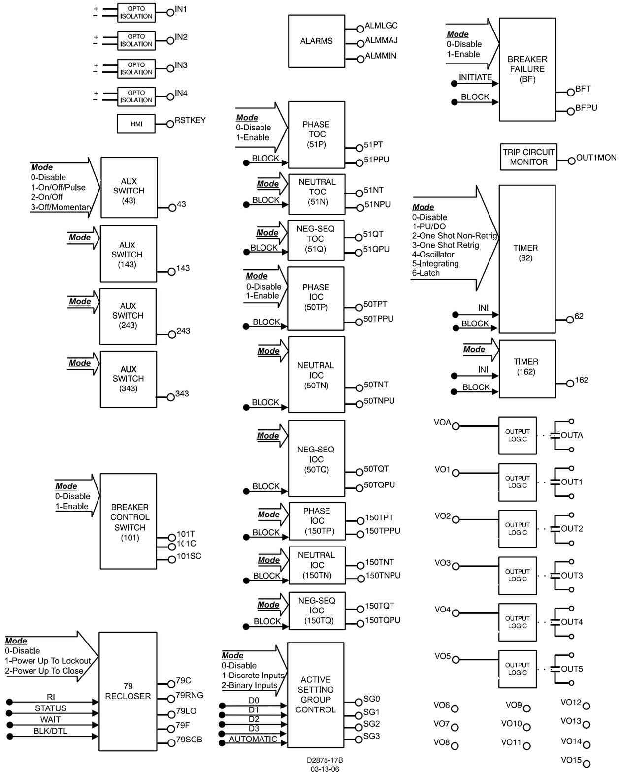
Figure 7-2. BESTlogic Sensing Input Type H Function Blocks
