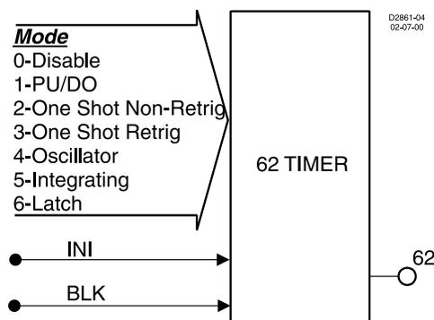
**Figure 4-21. General Purpose Logic Timers Logic Block**
