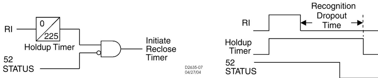
Figure 4-31. Recognition Dropout Timing
