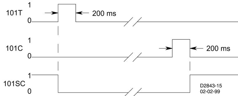
Figure 4-42. 101 Control Switch State Diagram
