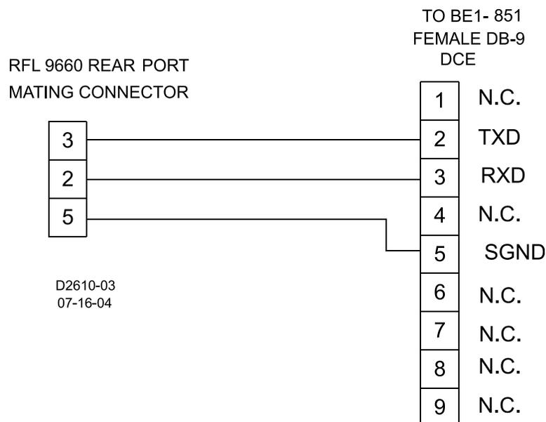
**Figure 12-21. RFL 9060 Protective Relay Switch to BE1-851 Cable**
