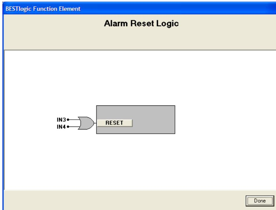
**Figure 6-21. BESTlogic Function Element Screen Alarm Reset Logic**
