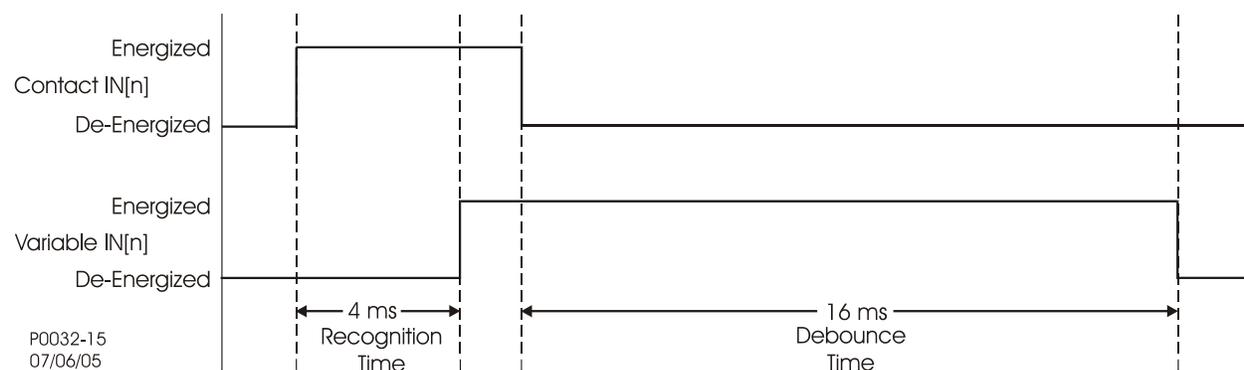
Figure 3-4. Digital Input Conditioning Diagram
