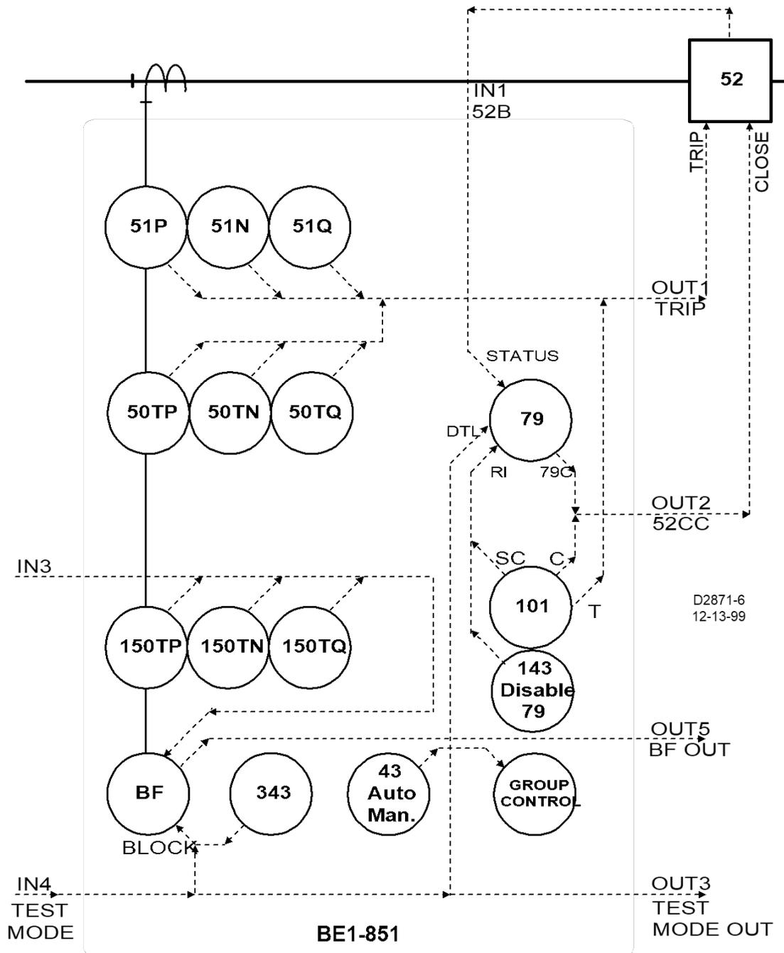
Figure 8-9. Typical One-Line Diagram for Feeder\_4 Logic
