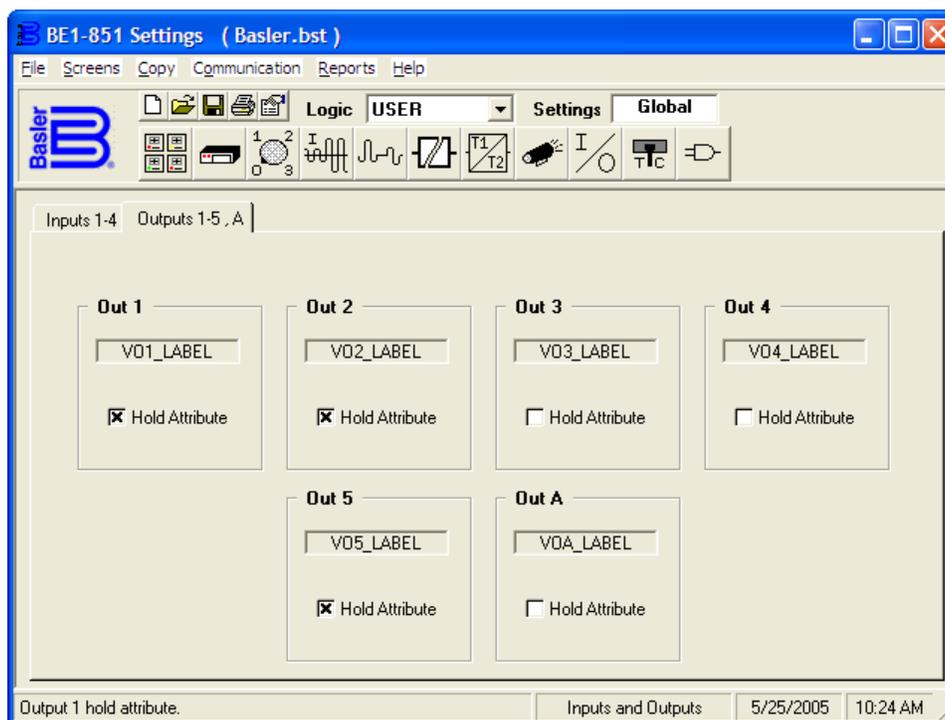
Figure 14-22. Inputs and Outputs Screen, Outputs 1 – 5, A Tab
