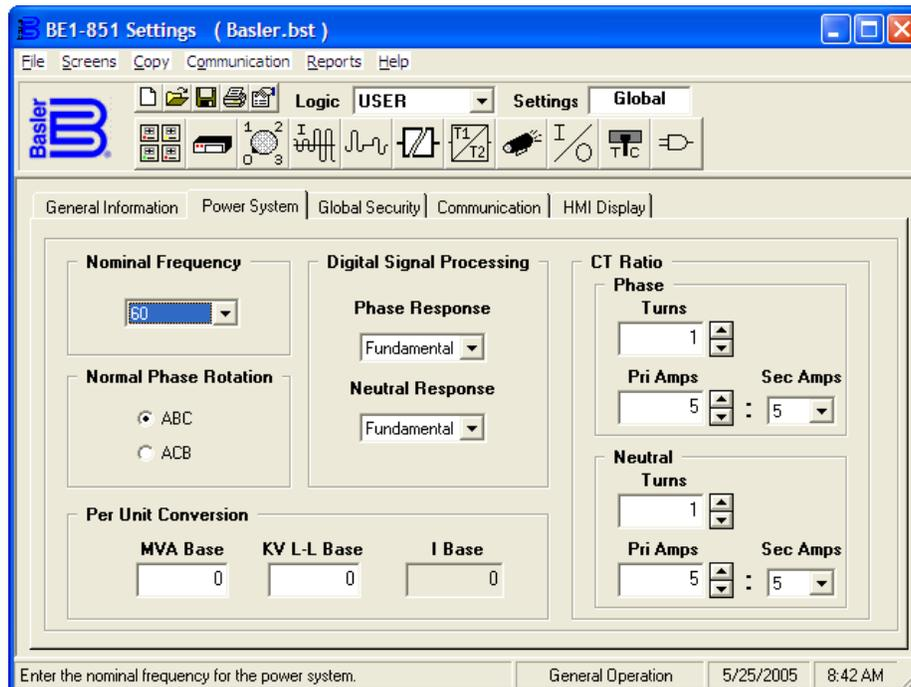
Figure 2-5. General Operation Screen, Power System Tab
