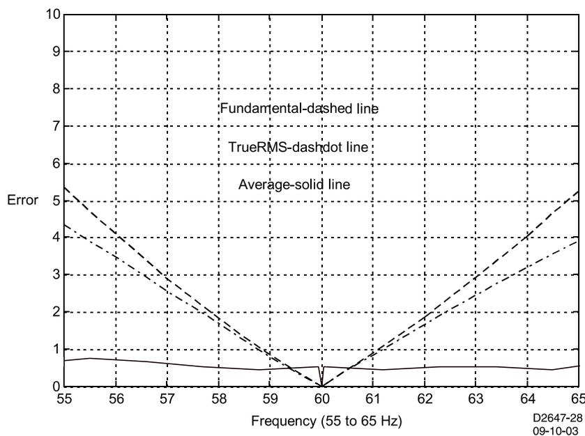
**Figure 3-1. Accuracy Characteristics, 55 to 65 Hz**
