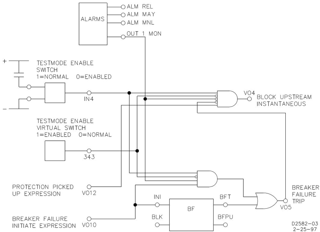
Figure 8-16. Trip Circuit Continuity and Voltage Monitor
