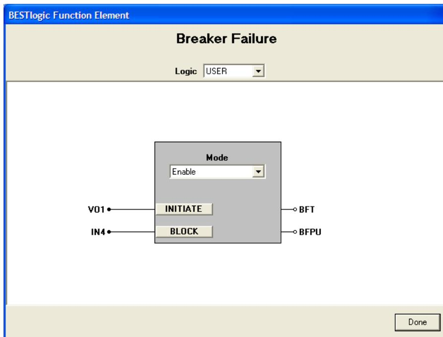
**Figure 4-19. BESTlogic Function Element Screen, Breaker Failure**
