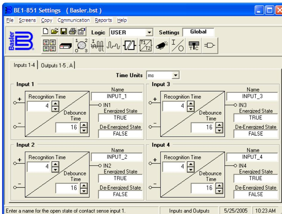
Figure 14-21. Inputs and Outputs Screen, Inputs 1 – 4 Tab
