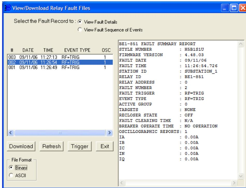
Figure 6-14. View/Download Relay Fault Files Screen
