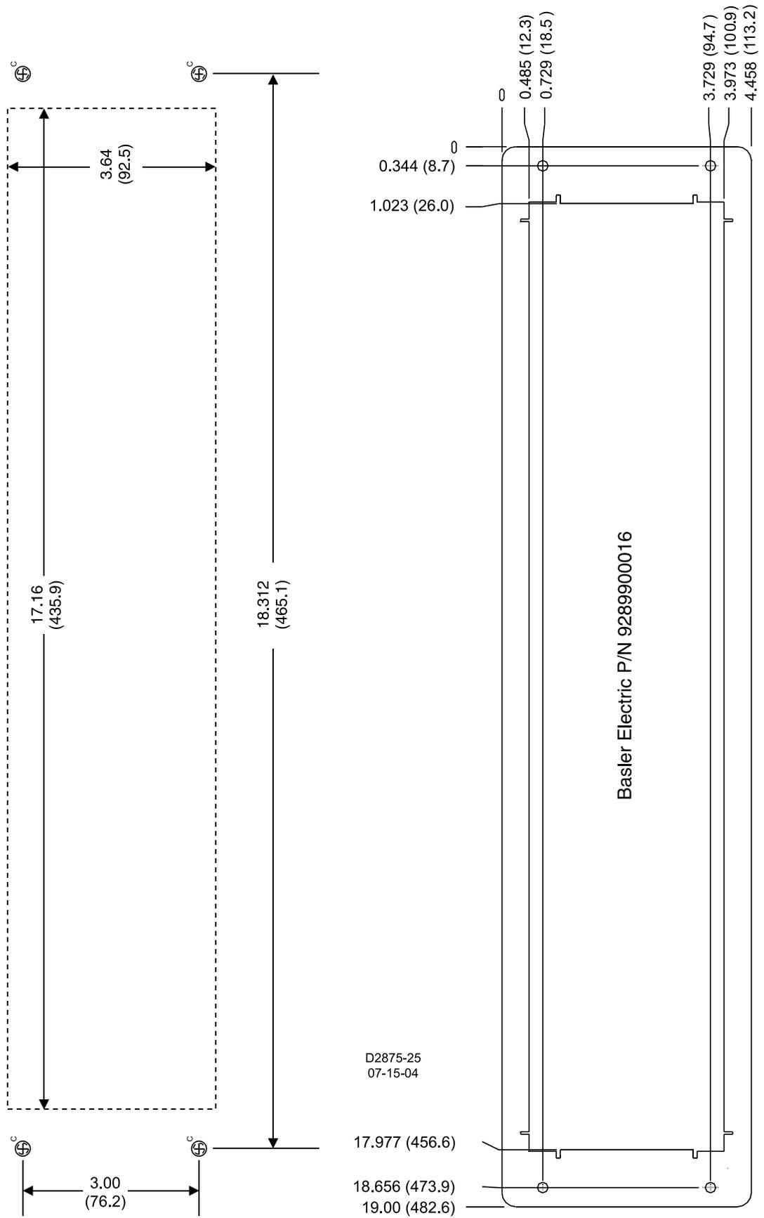
Figure 12-9. H1 Case, Two-Relay Mounting Plate Dimensions
