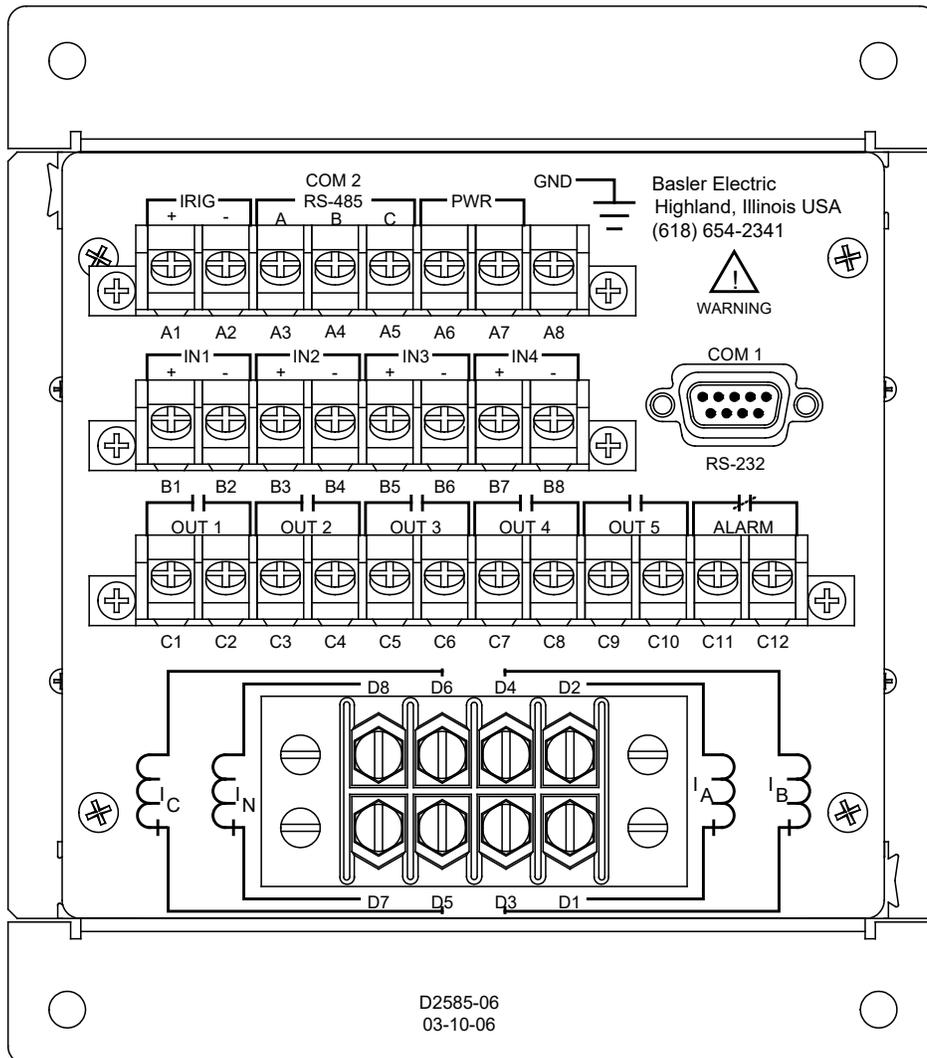
**Figure 12-16. F1 Case, Rear View, Terminal Connections**
