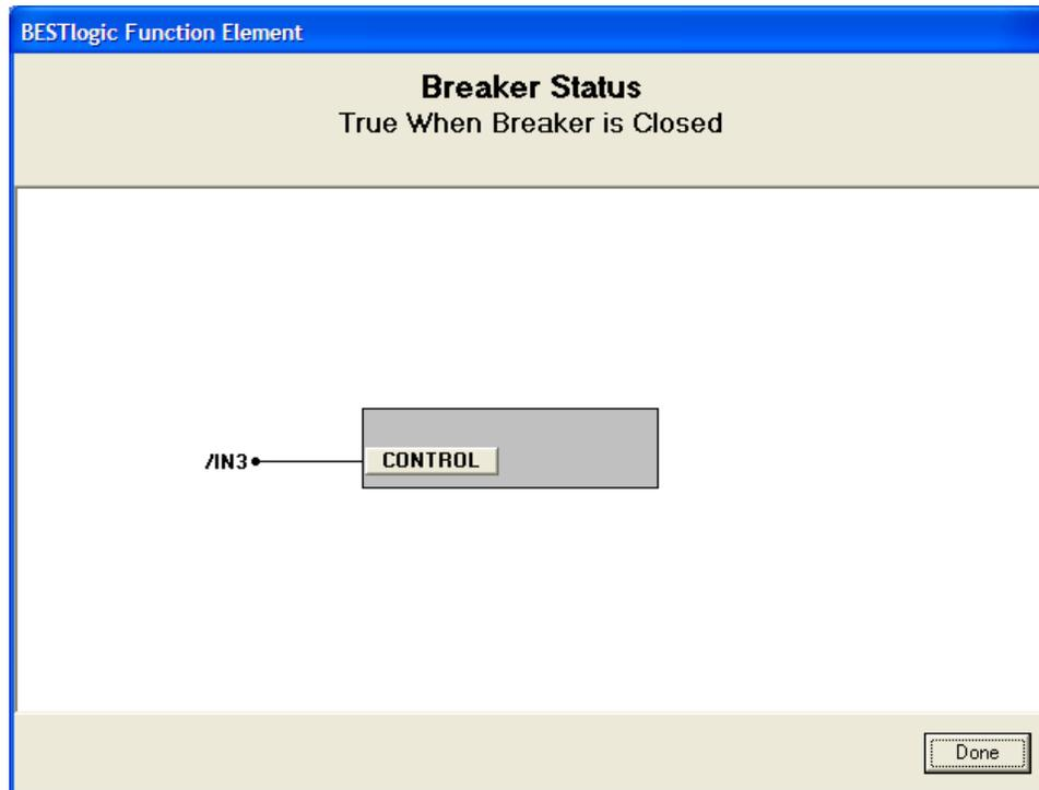
**Figure 6-4. BESTlogic Function Element Screen, Breaker Status**
