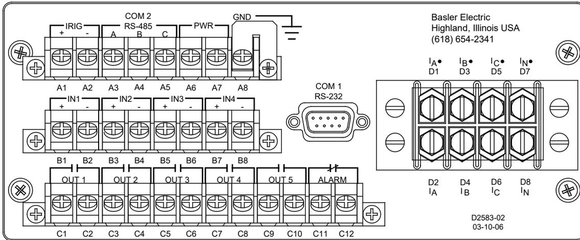
Figure 12-17. H1 Case, Rear View, Terminal Connections
