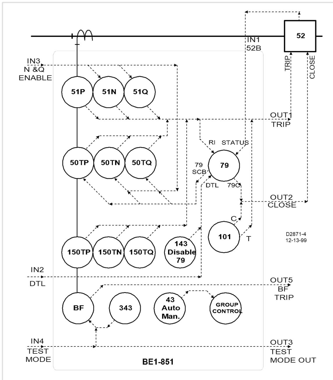
Figure 8-5. Typical One-Line Diagram for Feeder\_2 Logic
