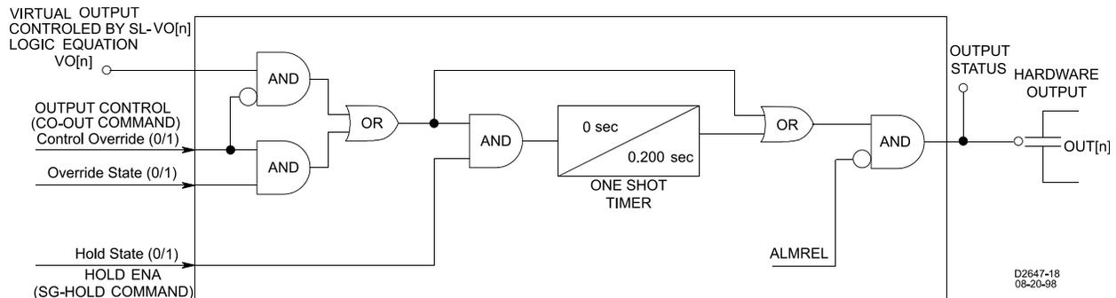
Figure 3-6. Output Logic, General Purpose Output Contacts
