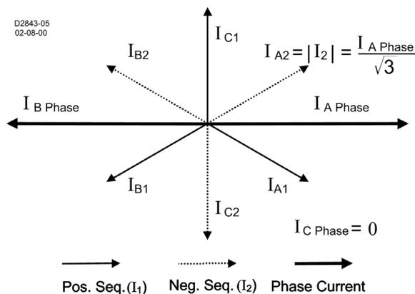
**Figure 4-17. Sequence Components for an A-B Fault**
