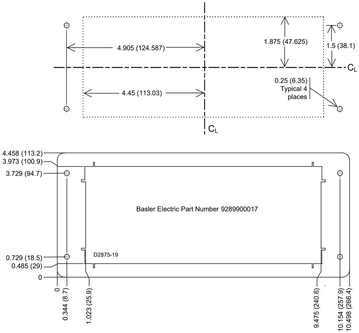
Figure 12-7. H1 Case, Single Relay Mounting Plate Dimensions
