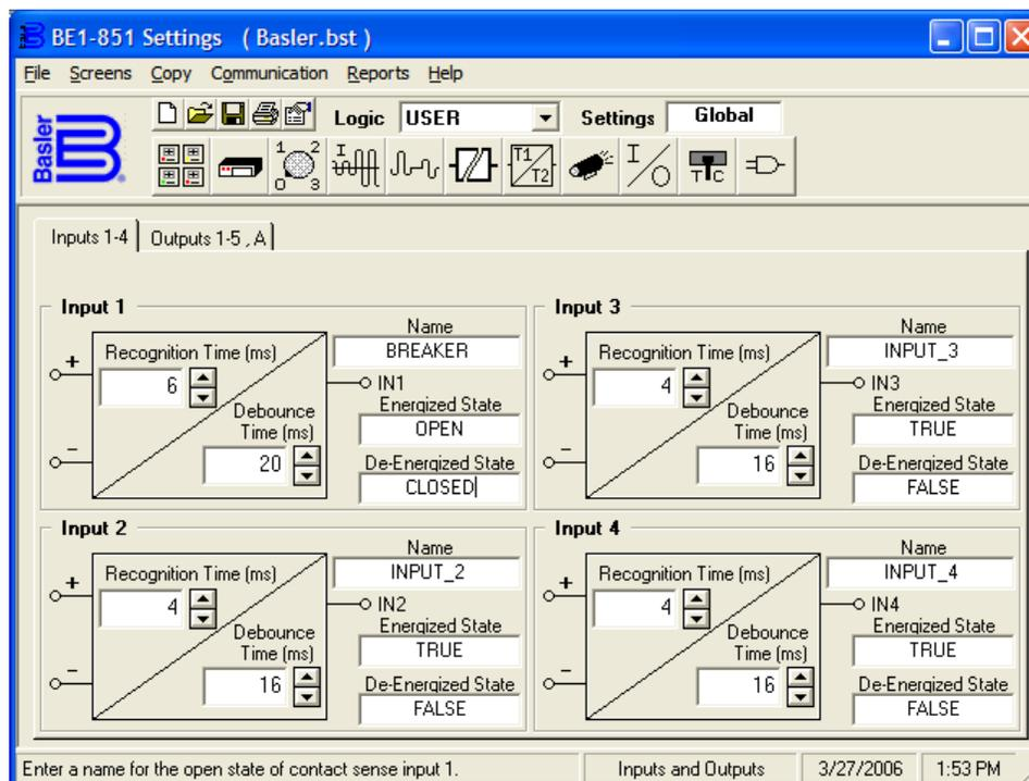
Figure 3-5. Inputs and Outputs Screen, Inputs 1-4 Tab
