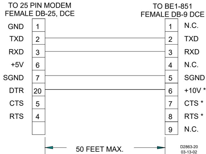
**Figure 12-23. Modem to BE1-851 (Null Modem Cable)**
