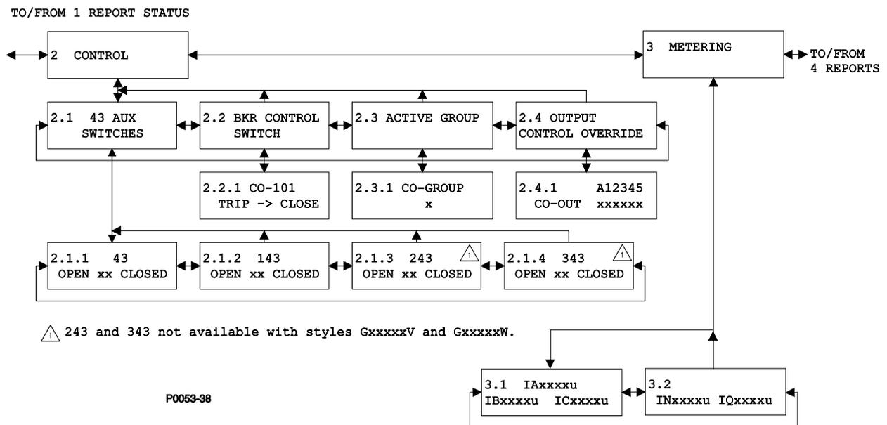
Figure 10-4. Control and Metering Branches Menu Tree
