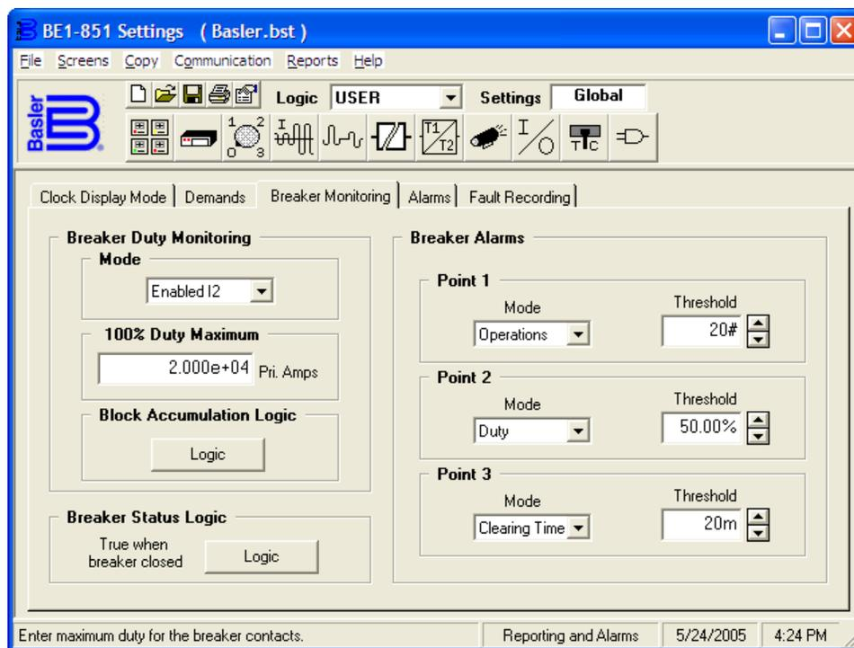
Figure 6-7. Reporting and Alarms Screen, Breaker Monitoring Tab
