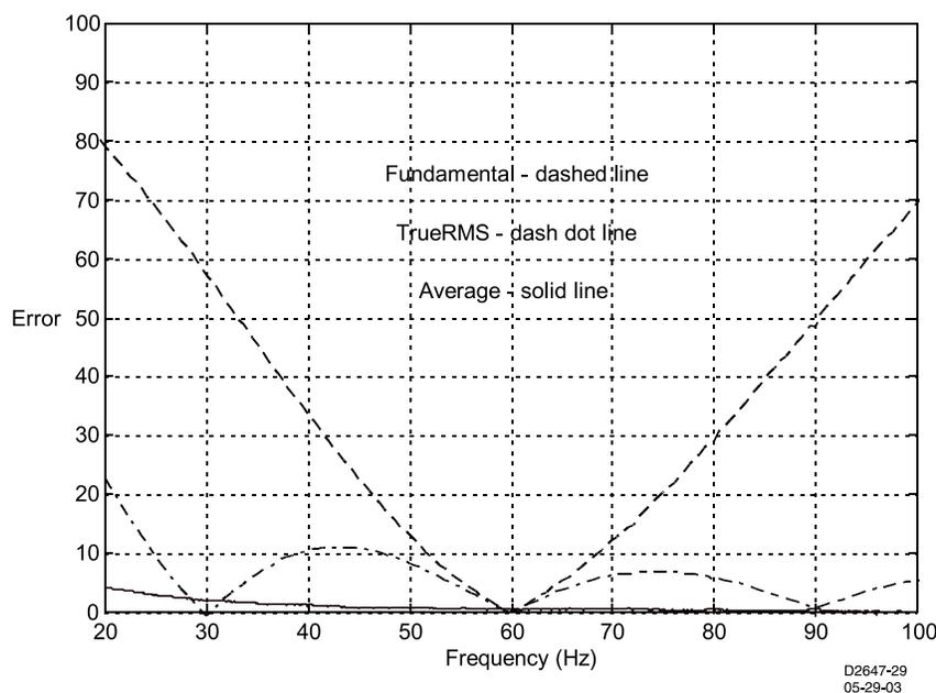
**Figure 3-2. Accuracy Characteristics, 20 to 100 Hz**
