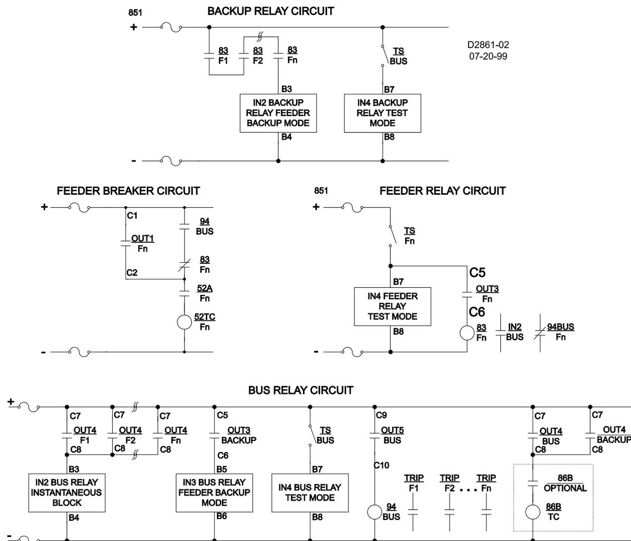
Figure 8-15. Interconnection Diagram for Integrated Protective System
