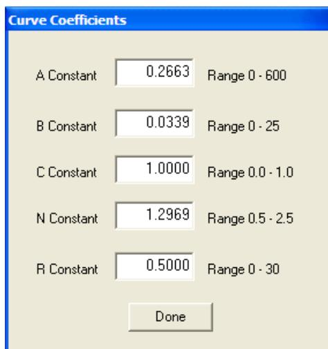
Figure 14-11. Curve Coefficients Screen
