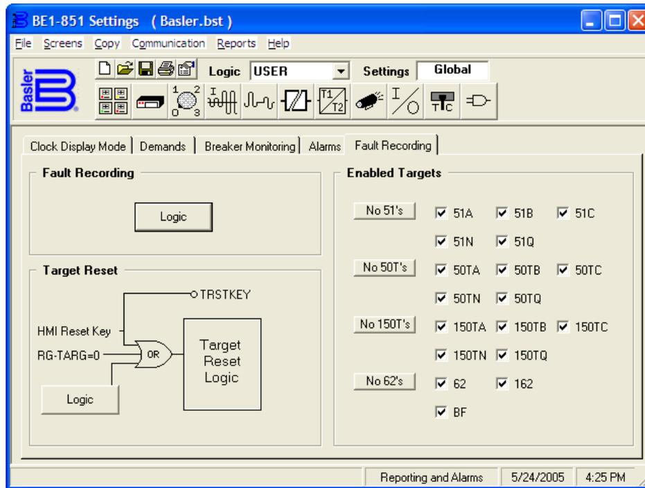
Figure 6-13. Reporting and Alarms Screen, Fault Recording Tab
