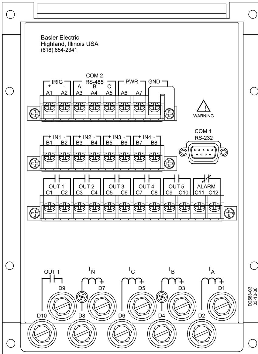
Figure 12-18. S1 Case, Rear View, Terminal Connections
