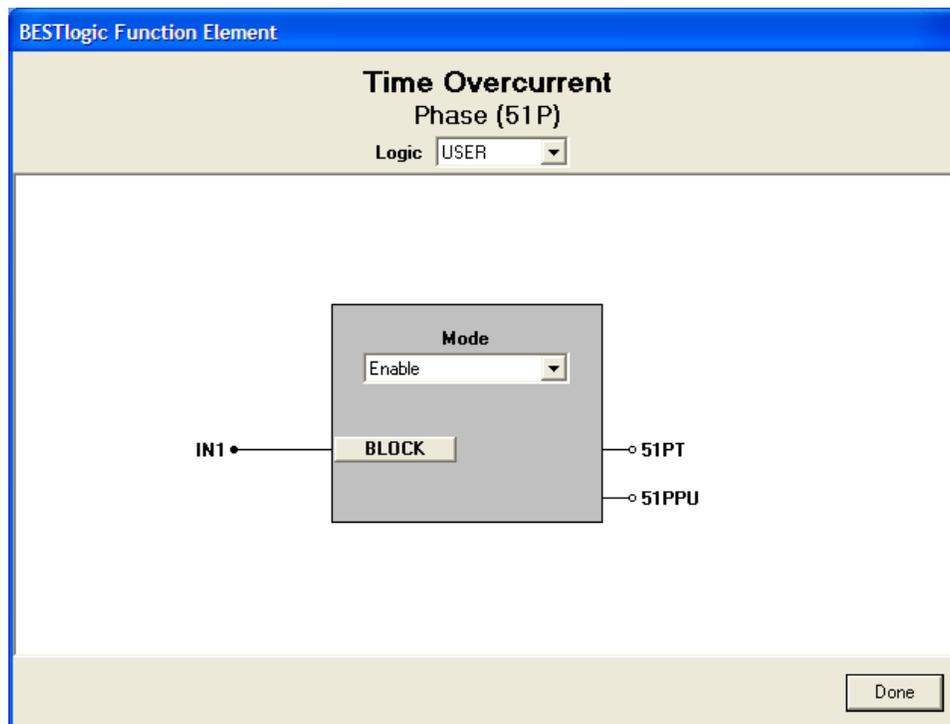
**Figure 4-13. BESTlogic Function Element Screen, Phase (51P)**
