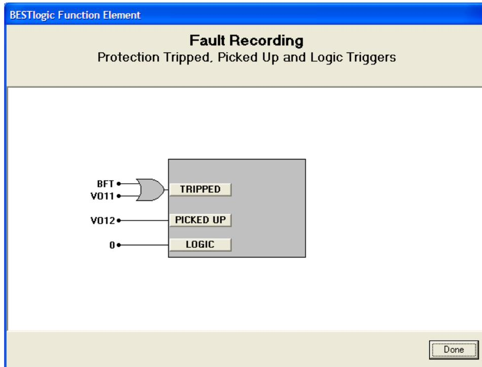
Figure 6-12. BESTlogic Function Element Screen, Fault Recording
