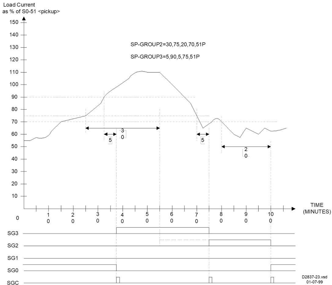
**Figure 4-6. Automatic Operation Based on Load Change**
