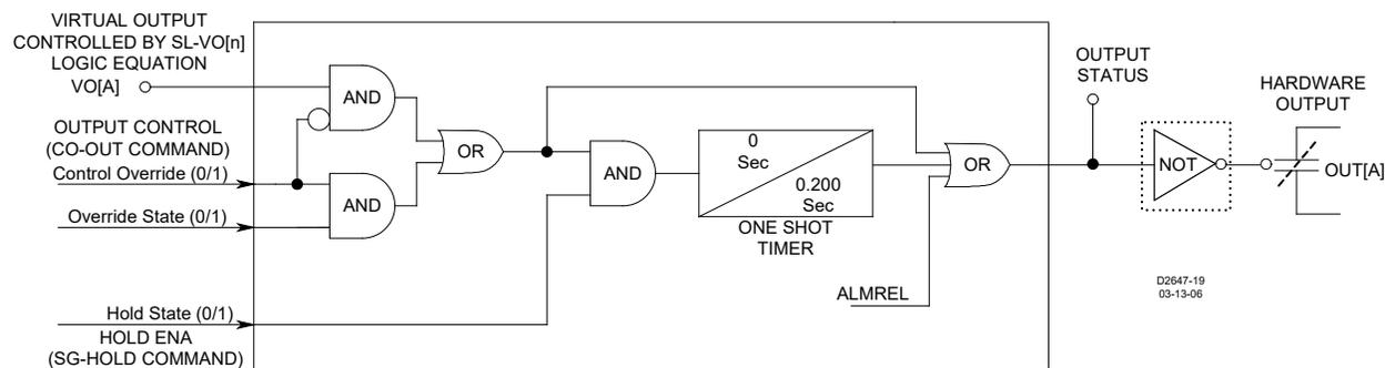
Figure 3-7. Output Logic, Fail-Safe Alarm Output Contact
