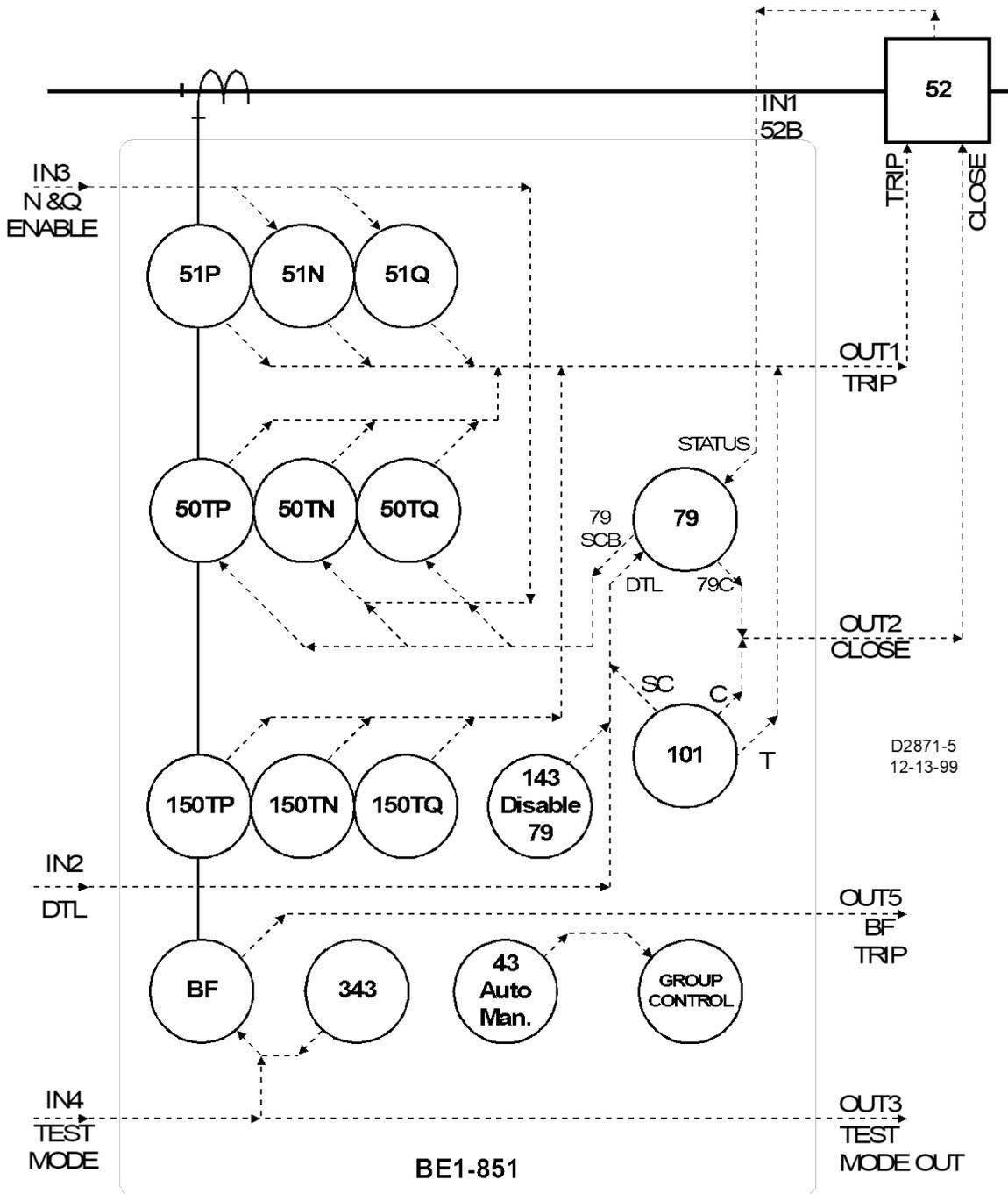
Figure 8-7. Typical One-Line Diagram for Feeder\_3 Logic
