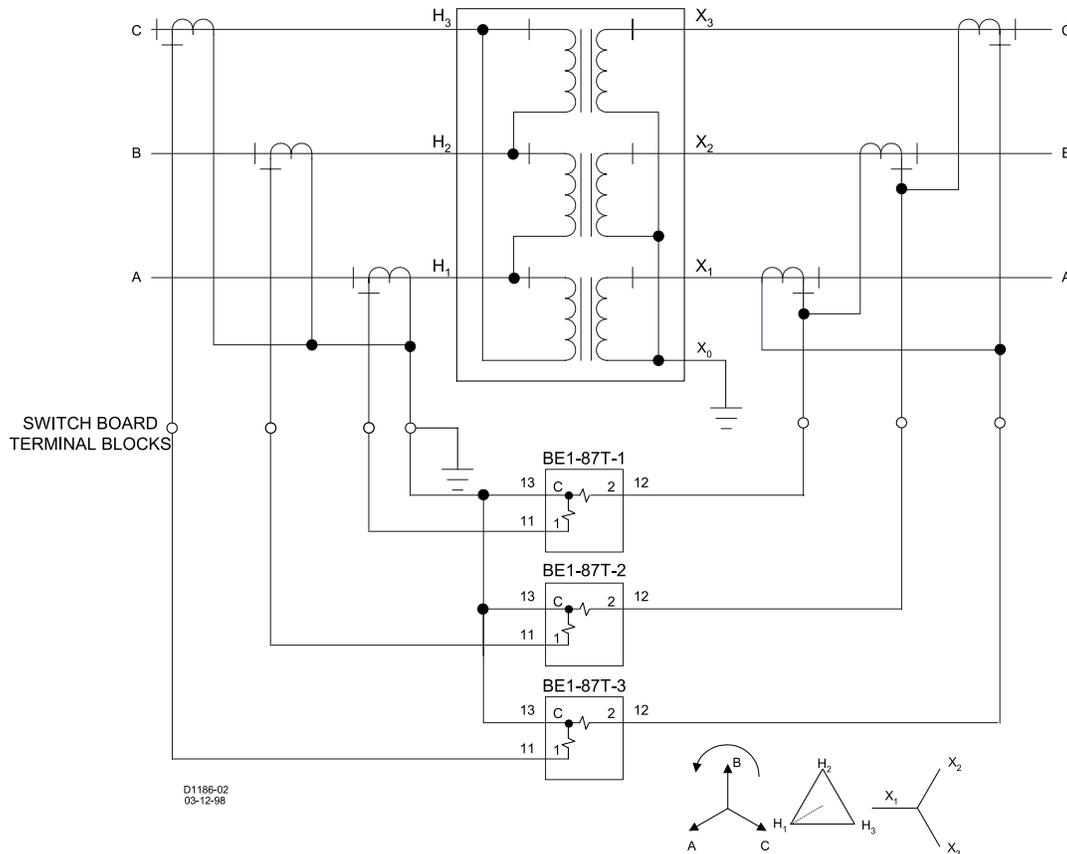
Figure 8 - Transformer Delta Compensation Using Delta CTs
