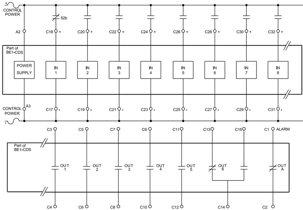
Figure 16b – BE1-CDS220, DC Connections
