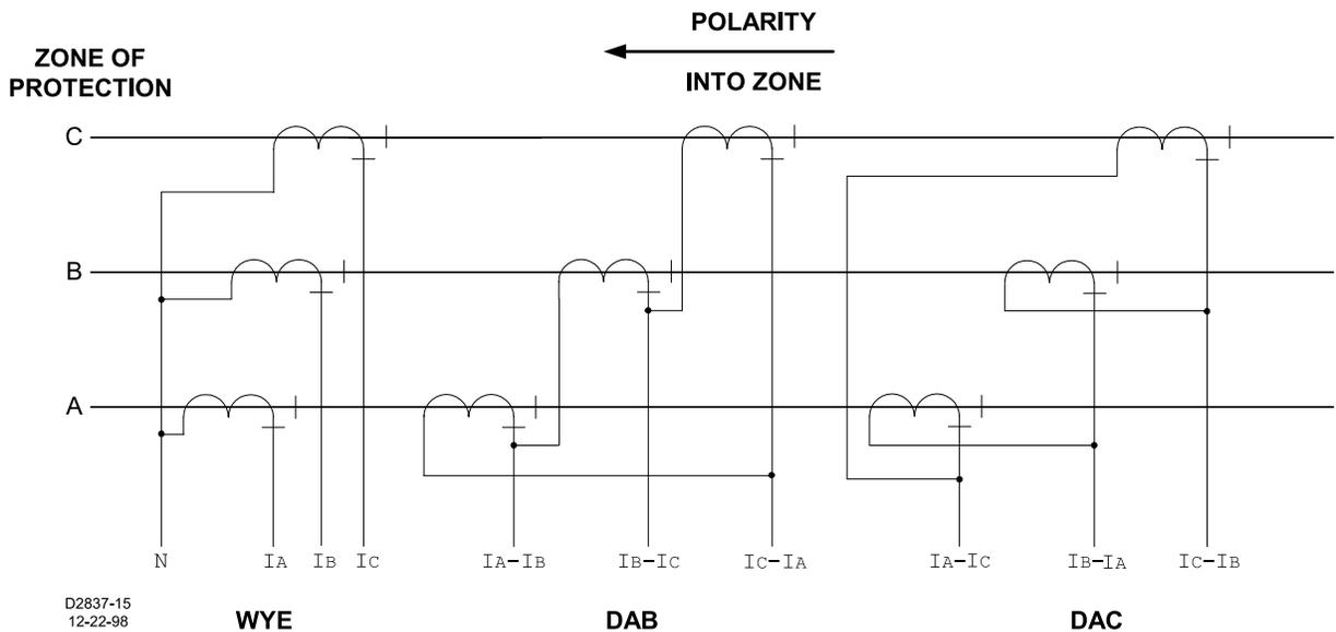
Figure 7 -  $D_{AB}$  vs.  $D_{AC}$  CT Connections
