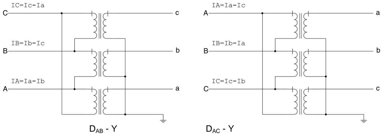
Figure 6 -  $D_{AB}$  vs.  $D_{AC}$  Transformer Connections (from Ref. 3)
