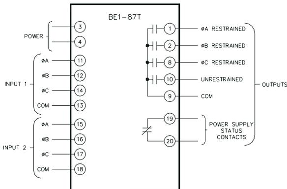
Figure 15c – BE1-87T, Three Phase, 2 Input, Output Option F
