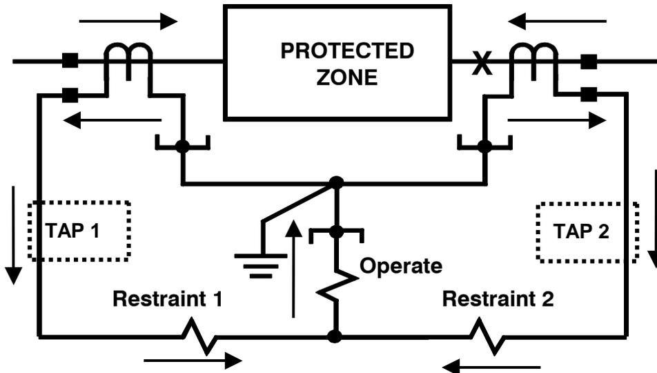
Figure 2 - Basic Differential Relay Concept
