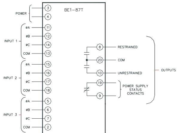
Figure 15d – BE1-87T, Three Phase, 3 Input, Output Option E
