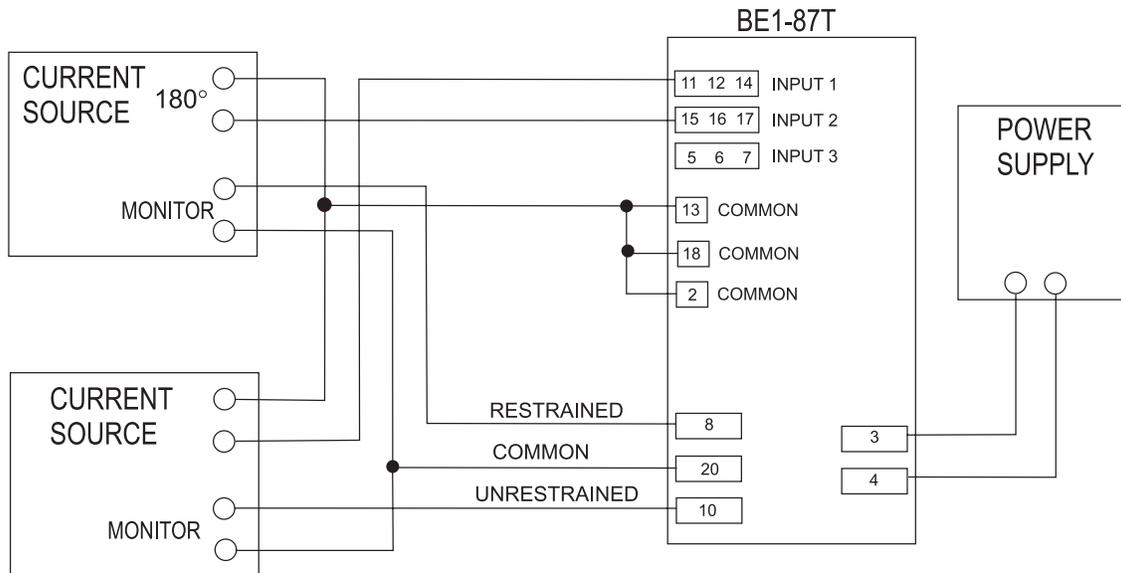
Figure 14 – BE1-87T, Three Phase, Sensing Input Type G, Output Option E
