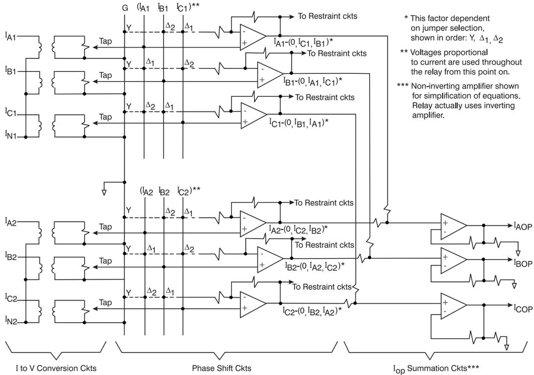
Figure 9 - The Delta Compensation Schemes of the BE1-87T
