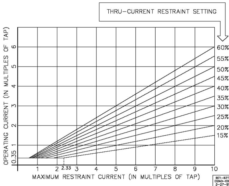
Figure 3 - Operate vs. Restraint and Minimum Operate, BE1-87T
