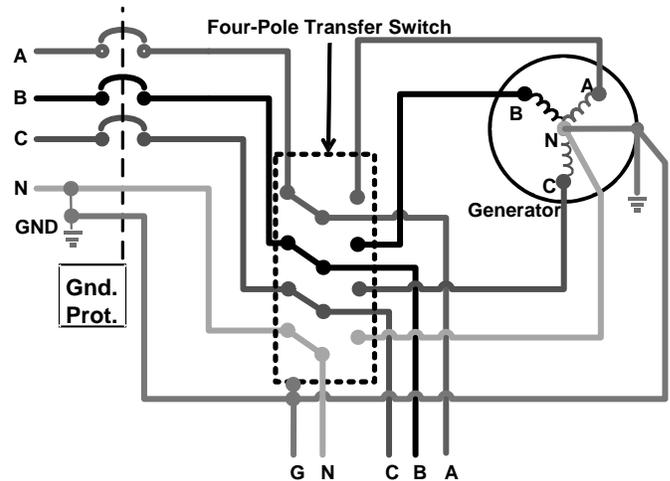
Fig. 6. Switching the Neutral with a Four-Pole Transfer Switch Gives Correct Currents to Ground Fault Protection
