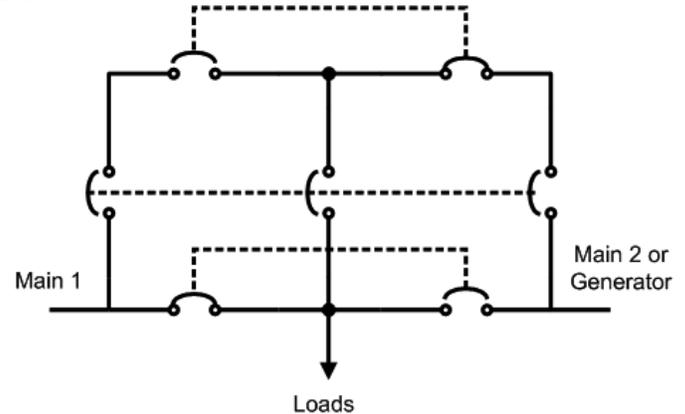
Fig. 7. Bypass Switch for Maintenance
