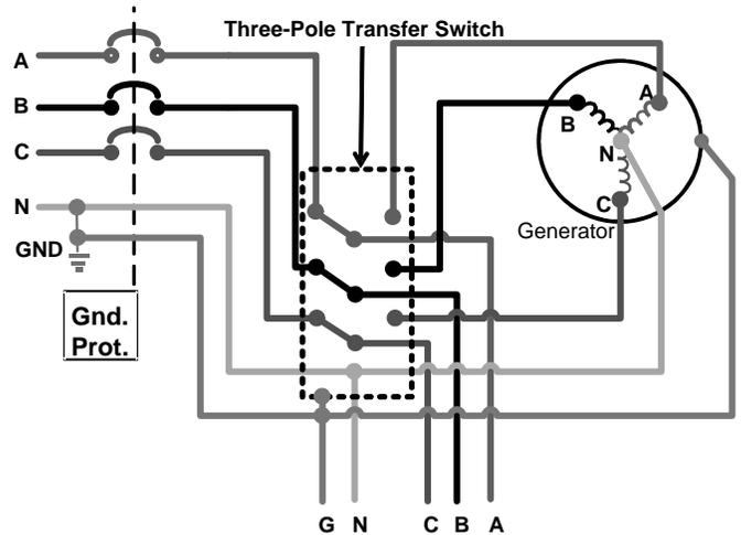
Fig. 3. Three-Pole Transfer Switch; Correctly Grounded Standby Power
