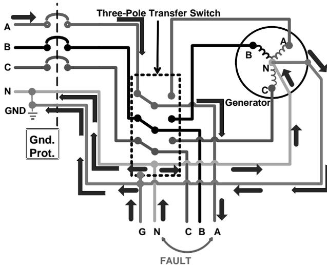
Fig. 5. Incorrectly Bonded Generator with A-N Fault
