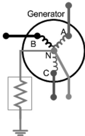
Fig. 2. Neutral to Ground Resistor for High-Resistance Grounding
