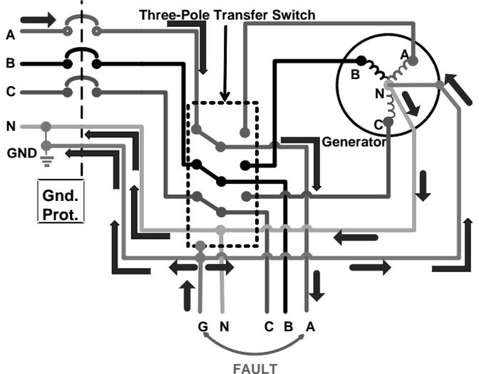
Fig. 4. Incorrectly Bonded Generator Neutral with Ground Fault
