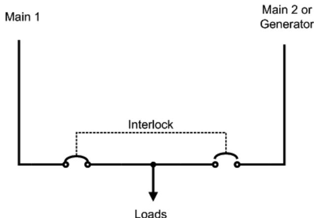
Fig.1. Basic Transfer Switch Operation
