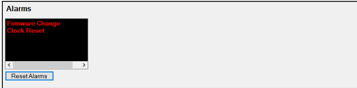
Figure 11-18. DECS-450 Alarm Annunciation and Reset Screen
