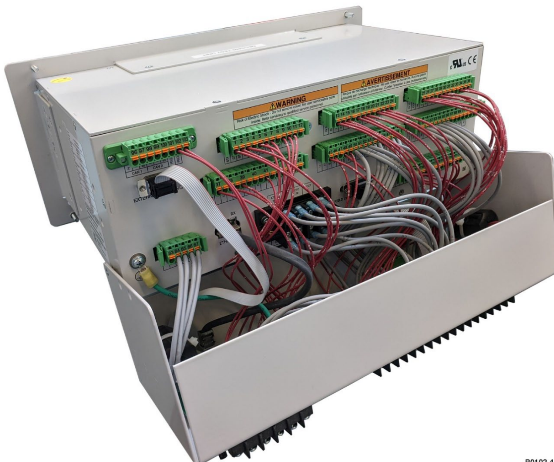
Figure 15-5. Transition Plate Wiring to DECS-450
